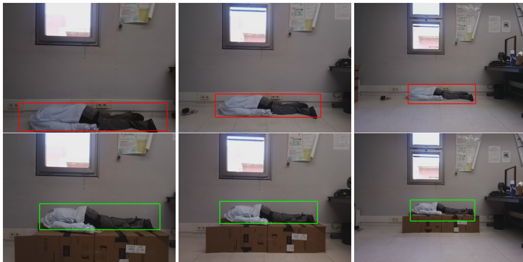
Figure 7. Fall/nonfall detection 1.5, 2 and 3 m away (each pair of images are in the same column).
