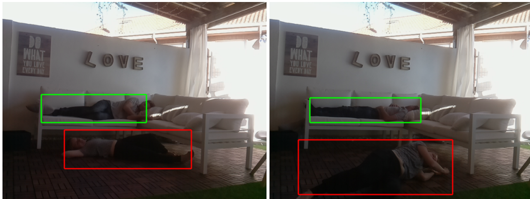
Figure 12. Example images from testing test where algorithm differentiates between fallen person and resting person.
