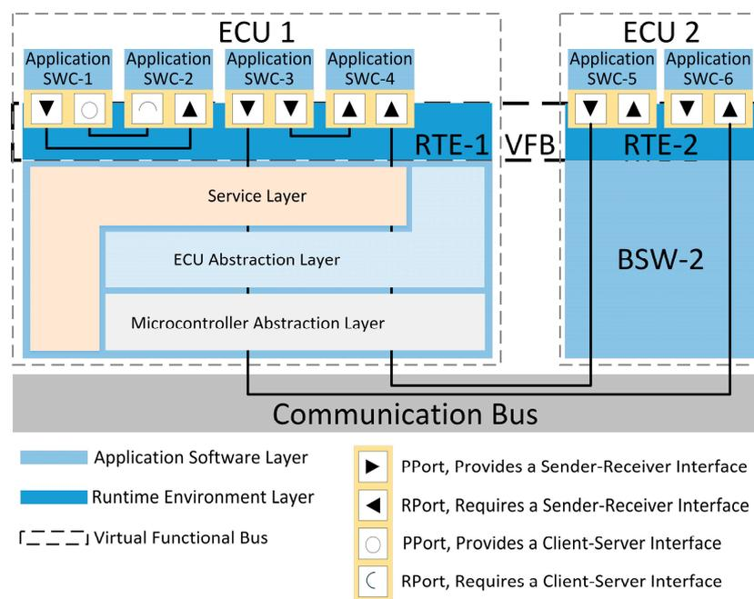
Figure 1. Simplified AUTOSAR software architecture.
