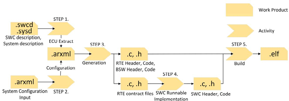
Figure 3. Open source AUTOSAR procedure.
