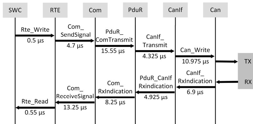
Figure 10. AUTOSAR controller area network (CAN) communication stack latency in each layer.
