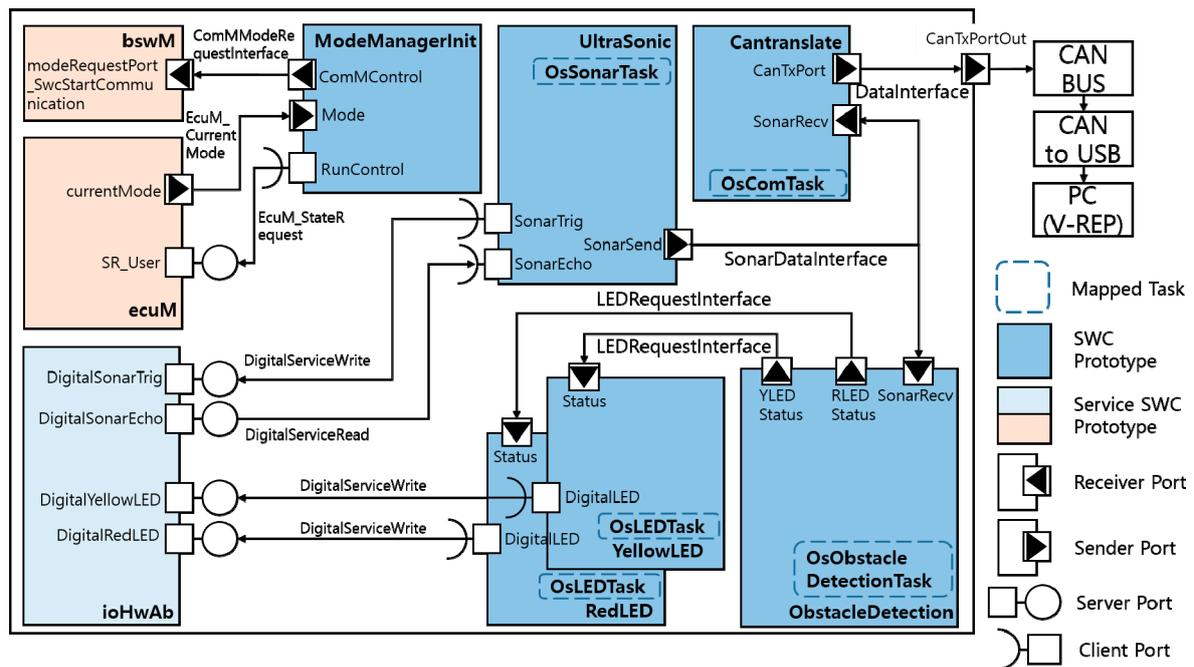
Figure 4. Collision warning application layer overview.
