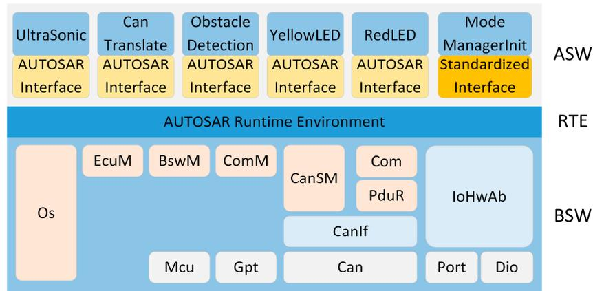
**Figure 5.** Layered collision warning system architecture.
