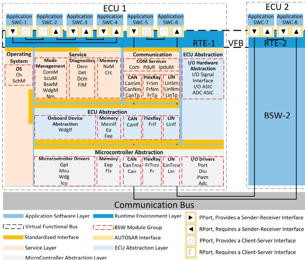
Figure 2. Detailed AUTOSAR software architecture.
