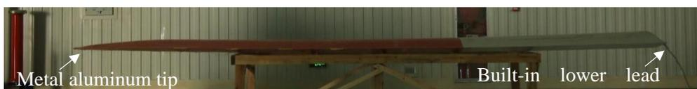
(b) 6 m and 1.5 MW wind turbine blade tip
