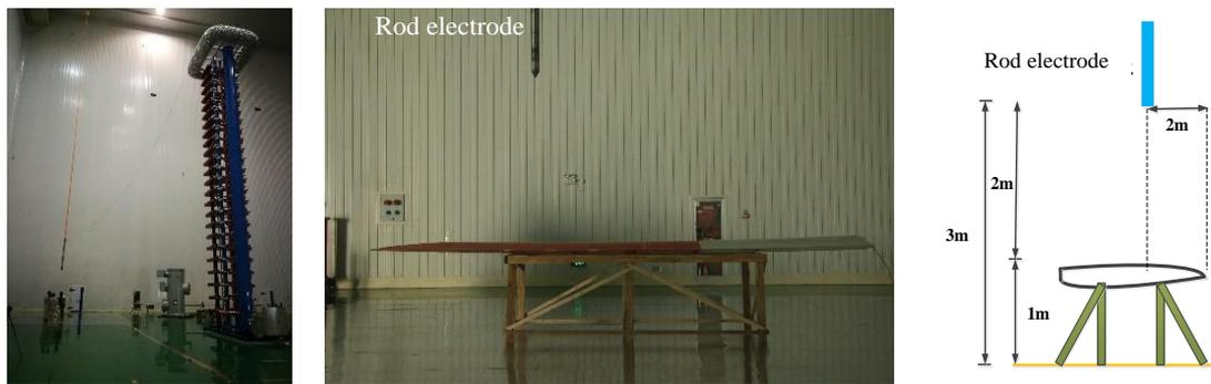
Figure 4. Experimental device.
