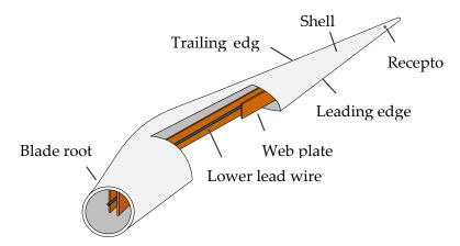
Figure 2. Lightning protection system recommended by IEC/TR 61400-24.
