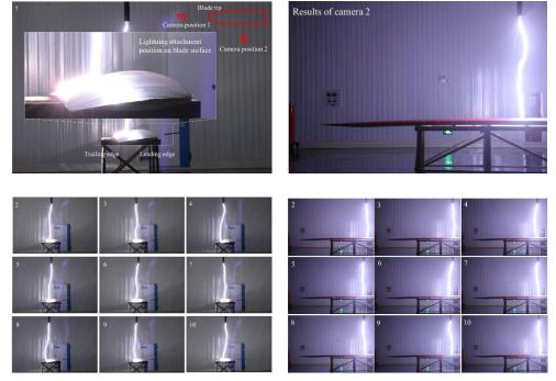
(a) Discharge test without the new lightning protection system (NLPS).
