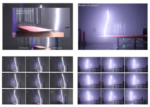
(b) Discharge test with the NLPS
