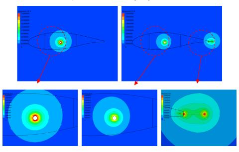
Figure 8. Cloud map of electric field intensity around the airfoil.
