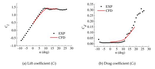
Figure 9. Lift coefficient curve (a), and drag coefficient curve (b) of DU93-W-210 airfoil.
