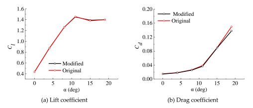
Figure 10. Aerodynamic performance comparison of the airfoil with and without the NLPS.
