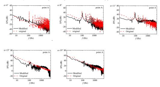
Figure 17. Sound pressure spectrum at monitoring point A.
