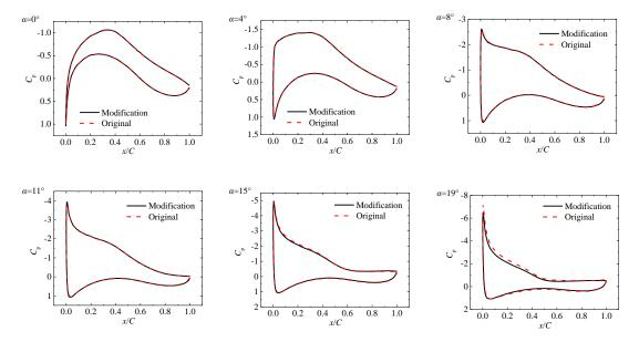
**Figure 11.** *C<sub>p</sub>* distribution of the airfoil with and without the NLPS.
