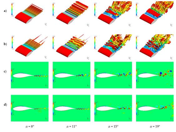
**Figure 15.** Isosurface of Q (**a**,**b**) and vorticity cloud diagram (**c**,**d**) at the symmetric plane. (**a**,**c**) are original; (**b**,**d**) are modified.
