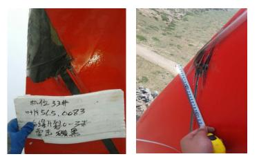
Figure 1. Lightning damage of wind turbine blades (Picture source: Blade manufacturers).
