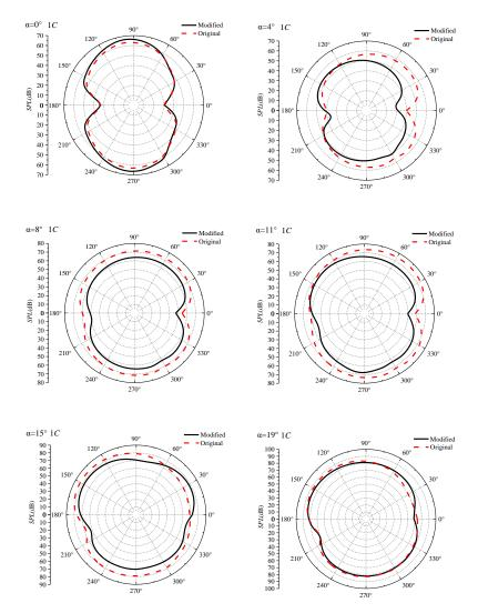
Figure 13. The directivity distribution of airfoil noise with and without the NLPS.
