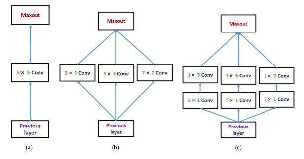
**Figure 3.** Proposed multi-scale inception block of two successive convolutions [53]. (**a**) Single Scale Convolution (**b**), Multi-Scale Convolution, and (**c**) proposed.
