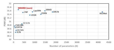
**Figure 5.** The model complexity comparison in number of parameters versus PSNR [56]. The performance of model complexity are evaluated on Set5 [56] dataset for  $4 \times$  SR [67].
