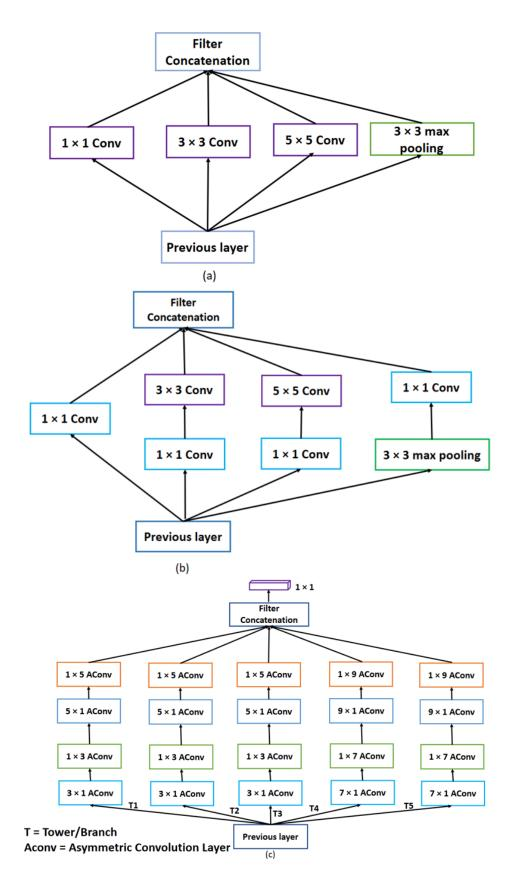
**Figure 4.** Inception block with different towers [54] used for multi-scale reconstruction stage-II. (a) Inception module, naive version; (b) inception module with dimension reductions [55]; and (c) our proposed module.
