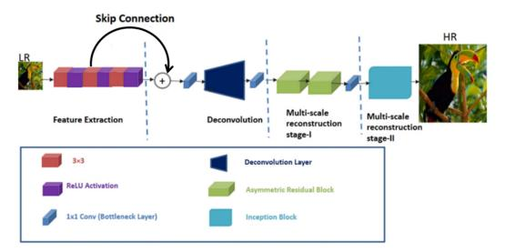
**Figure 1.** The complete network architecture of our proposed super-resolution (SR) method. Our network consists of feature extraction, deconvolution, multi-scale reconstruction stage-I, and multi-scale reconstruction stage-II. LR = low-resolution; HR = high-resolution; ReLU = rectified linear unit; Conv = convolution.
