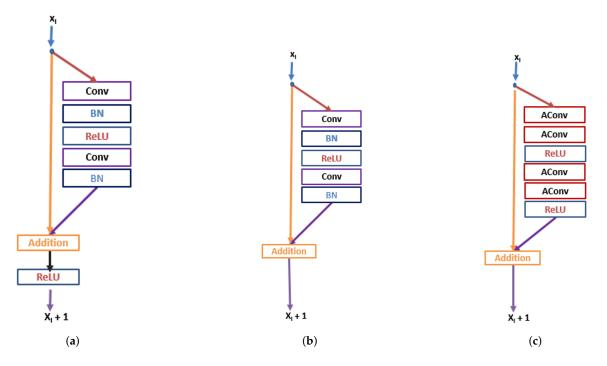
**Figure 2.** The comparison design of residual connection blocks [49] with our proposed residual block. (a) Original residual neural network (ResNet) [34]. (b) SRResNet [19]. (c) Proposed. BN = batch normalization; AConv = asymmetric convolution.
