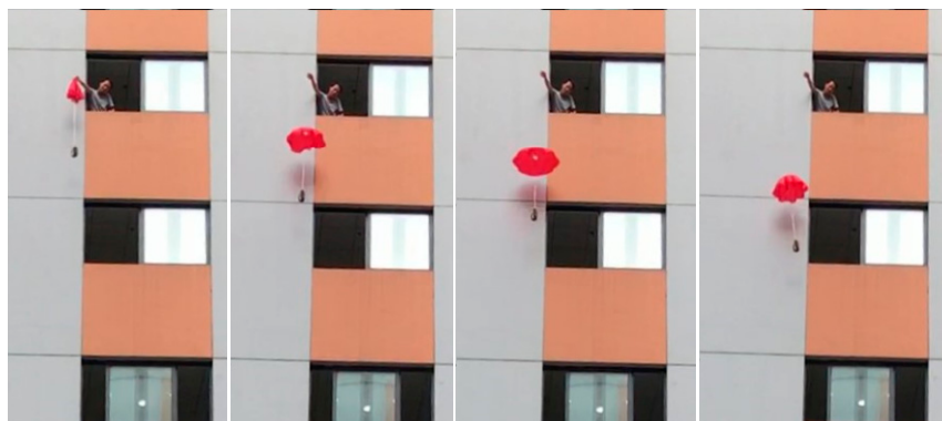
Figure 5. The opening process of the parachute in the airdropped experiment.
