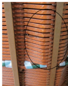
Figure 22. Artificial winding deformation: Radial buckling of the A phase winding after short-circuit.
