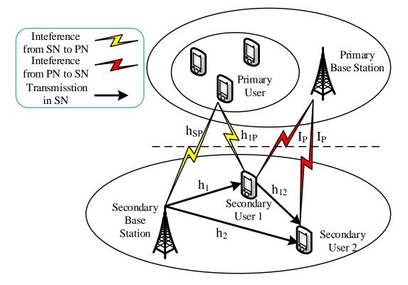
**Figure 1.** System model of cognitive radio(CR) and section scheme of OMA/non-orthogonal multiple access(NOMA).
