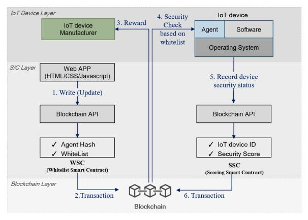
**Figure 1.** Security level evaluation mechanism for extending the Internet of things (IoT) networks based on a blockchain.
