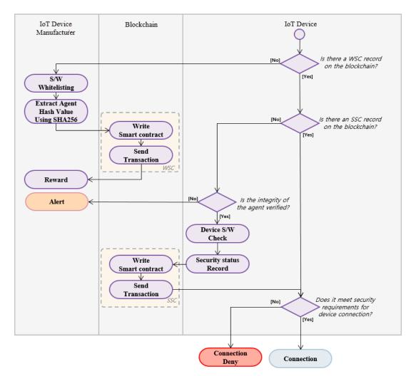
Figure 2. Flowchart for the proposed secure IoT extension.
