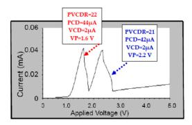
Figure 10. I-V curve of practical double PVCDR RTEC structure.
