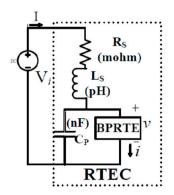
Figure 3. Single PVCDR RTEC unit with C<sub>p</sub>, R<sub>S</sub> and L<sub>S</sub> values [1].
