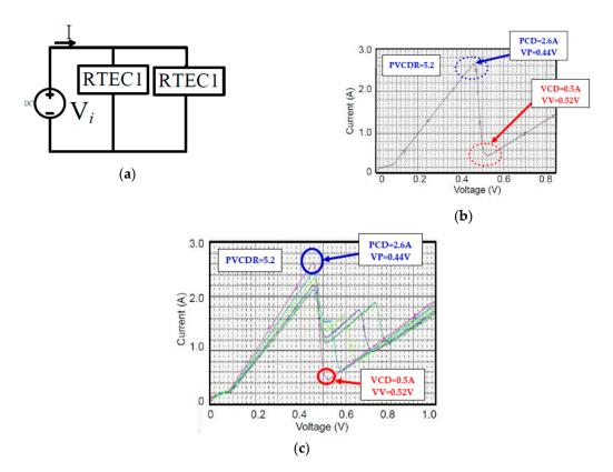
**Figure 5.** (**a**) Paralleled structure of two PVCDR RTEC units. (**b**) Single NDR curve of paralleled structure of two PVCDR RTEC units with PCD value of 2.6 A. (**c**) Double NDR curve of double PVCDR RTEC structure with variable *R*<sub>S</sub>.
