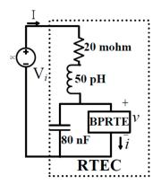
**Figure 4.** Optimum single PVCDR RTEC equivalent circuit with  $C_p$  of 80 nF,  $R_S$  of 20 m $\Omega$  and  $L_S$  of 50 pH values [1].
