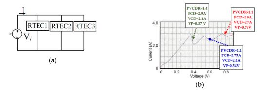
**Figure 8.** (a) The construction of triple PVCDR RTEC structure. (b) NDR curve of triple PVCDR RTEC structure.
