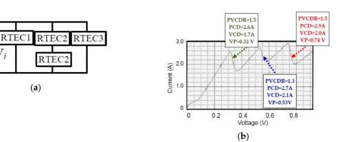
**Figure 9.** (a) The equivalent circuit of triple PVCDR RTEC structure with adding the fourth RTEC unit. (b) Symmetry NDR characteristic of triple PVCDR RTEC structure with adding the fourth RTEC unit.
