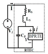
Figure 1. Scheme of basic resonant tunneling electronic circuit (RTEC) unit [1].
