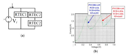
**Figure 7.** (**a**) The second improvement method by the double PVCDR RTEC structure in series with another RTEC unit. (**b**) Improvement of NDR characteristic by the method of the double PVCDR RTEC structure in series with another RTEC unit.
