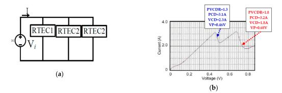
**Figure 6.** (a) Improvement of double PVCDR RTEC structure by paralleled the third RTEC unit. (b) Improvement of NDR characteristic with different and asymmetry PVCDR values after paralleled another same single PVCDR RTEC unit.
