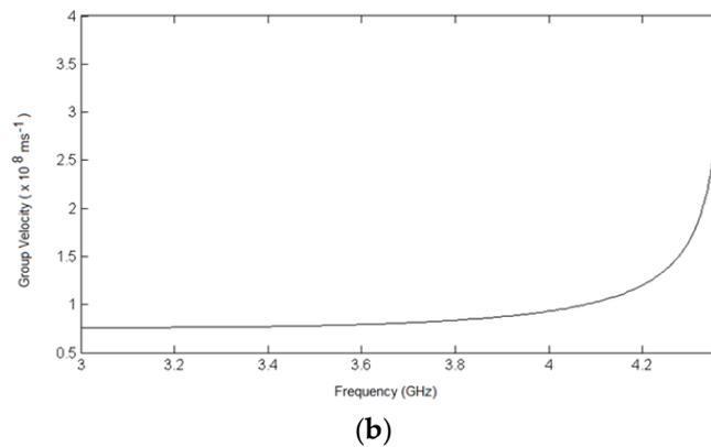
**Figure 2.** Details of the experiment. **(a)** The photo showing the actual measurement setup for measuring the blood glucose on the left hand; and **(b)** calculated group velocity of a surface wave propagating in the curved Goubau line (of which the diameter of the central conductor is 1 mm and the thickness of the gelatin coating is 3.8 mm).
