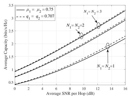
**Figure 8.** Average channel capacity using ORA technique of dual-hop relaying systems operating over  $\kappa - \mu$  shadowed fading links and its equivalent Nakagami-*q* fading links for different number of antennas.
