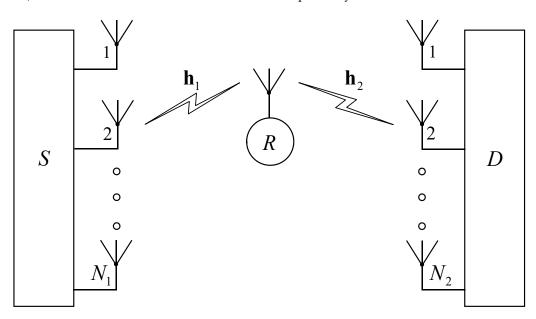
Figure 1. Dual-hop DF relaying system with beamforming.
