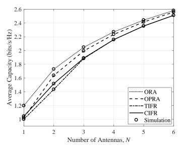
**Figure 5.** Average channel capacity of four adaptive transmission policies for different arrangements of antennas, *N* (*N*<sub>1</sub>, *N*<sub>2</sub>), when  $\overline{\gamma}_1 = \overline{\gamma}_2 = 8$  dB,  $\kappa_1 = \kappa_2 = 1$ ,  $\mu_1 = \mu_2 = 1$ , and  $m_1 = m_2 = 1$ .
