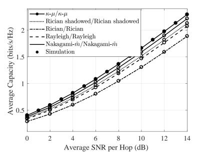
**Figure 4.** Average channel capacity of OPRA scheme for some channel models, viz., the Rician (when  $K_1 = K_2 = 5$ ),  $\kappa - \mu$  (when  $\kappa_1 = \kappa_2 = 4$  and  $\mu_1 = \mu_2 = 2$ ), Rician-shadowed (when  $K_1 = K_2 = 8$  and  $m_1 = m_2 = 0.5$ ), Rayleigh fading, and Nakagami- $\hat{m}$  (when the shaping factor of the Nakagami- $\hat{m}$  is set to 2 for each link).
