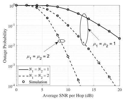
**Figure 2.** Outage probability against average SNR per hop for different arrangements of antenna and fading parameter  $\mu$  when  $\kappa_1 = \kappa_2 = 1$ ,  $m_1 = m_2 = 2$ , and  $\gamma_{th} = 10$  dB.
