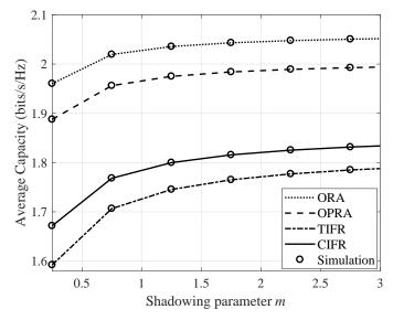
**Figure 6.** Average channel capacity under different adaptive transmission techniques for different shadowing parameter,  $m(m_1, m_2)$ , when  $\overline{\gamma}_1 = \overline{\gamma}_2 = 10$ ,  $N_1 = N_2 = 2$ ,  $\kappa_1 = \kappa_2 = 1$ , and  $\mu_1 = \mu_2 = 1$ .
