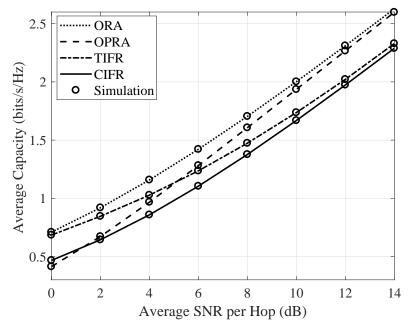
**Figure 3.** Average channel capacity for four different adaptive transmission methods with respect to the average SNR per hop when  $m_1 = m_2 = 0.5$ ,  $\mu_1 = \mu_2 = 1$ ,  $\kappa_1 = \kappa_2 = 1$ , and  $N_1 = N_2 = 2$ .
