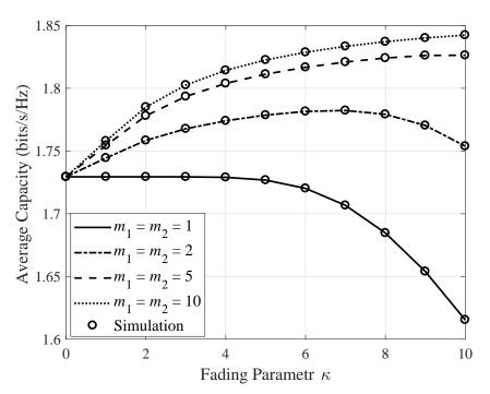
**Figure 7.** Average channel capacity of ORA technique with respect to the fading parameter  $\kappa$  ( $\kappa_1$ ,  $\kappa_2$ ) for different shadowing parameter *m* when  $\overline{\gamma} = 8$  dB,  $\mu_1 = \mu_2 = 1$ , and  $N_1 = N_2 = 2$ .
