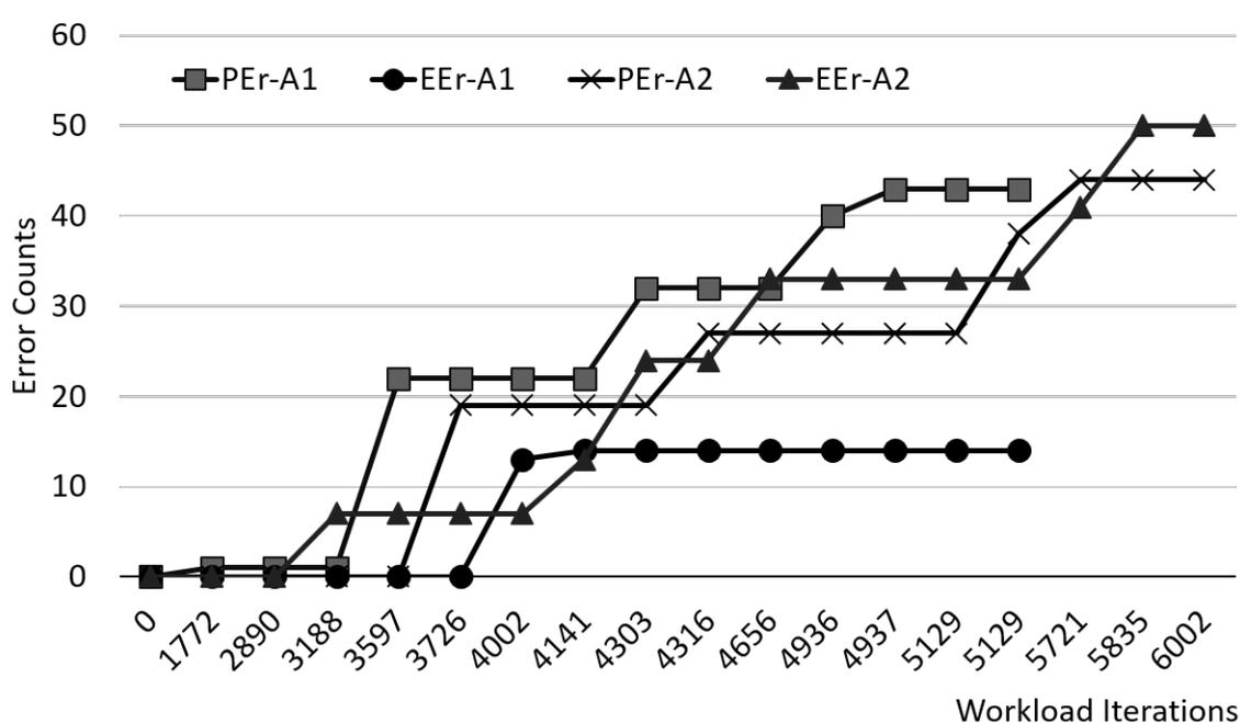
**Figure 4.** Trend of PEr and EEr during the whole lifetime of A1 and A2. **PEr-A1:** program error count of A1; **EEr-A1:** erase error count of A1; **PEr-A2:** program error count of A2; **EEr-A2:** erase error count of A2; **X axis:** pinpoint workload iteration of error occurrence; intervals are not uniformed.
