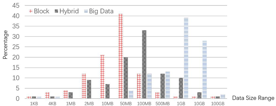
**Figure 2.** Distribution of data sizes under three workloads. The X axis is the data size range. For example, 4 KB includes data sizes ranging from 1 KB–4 KB. The Y axis is the percentage of each data size range.
