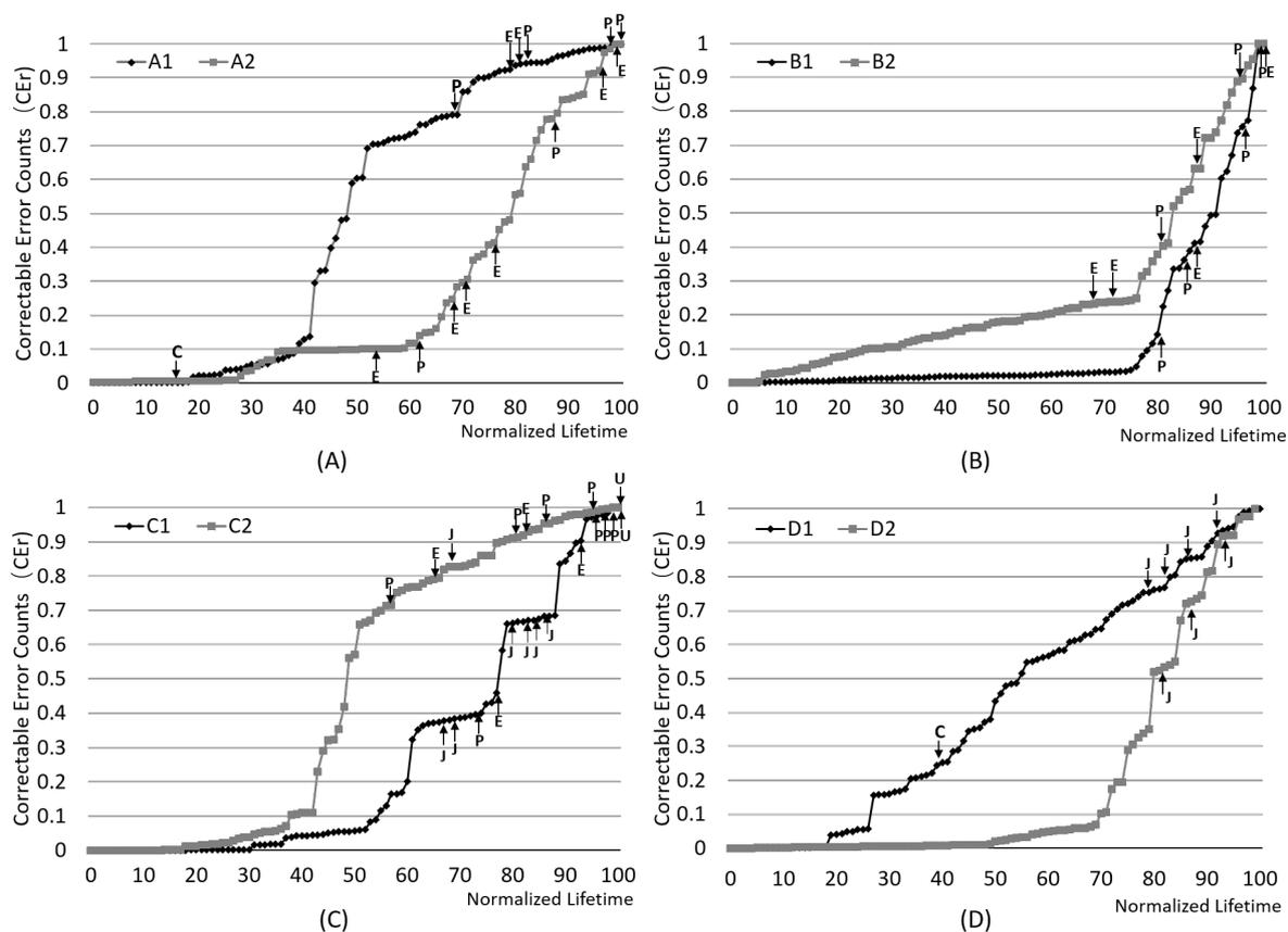
**Figure 5.** Trend of CEr during the whole lifetime of eight drives (e.g., A1 and A2 in (A)). P and E mean the surging of Program errors and Erase errors, respectively. U indicates the occurrence of Uncorrectable error. J and C correspondingly indicate the occurrence of performance Jitter and CRC error.
