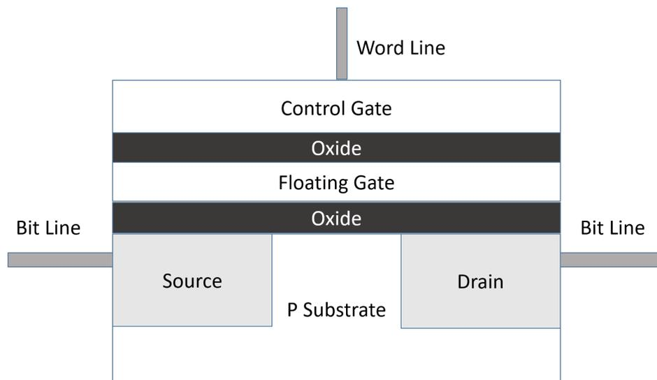
**Figure 1.** The structure of an NAND flash memory cell.
