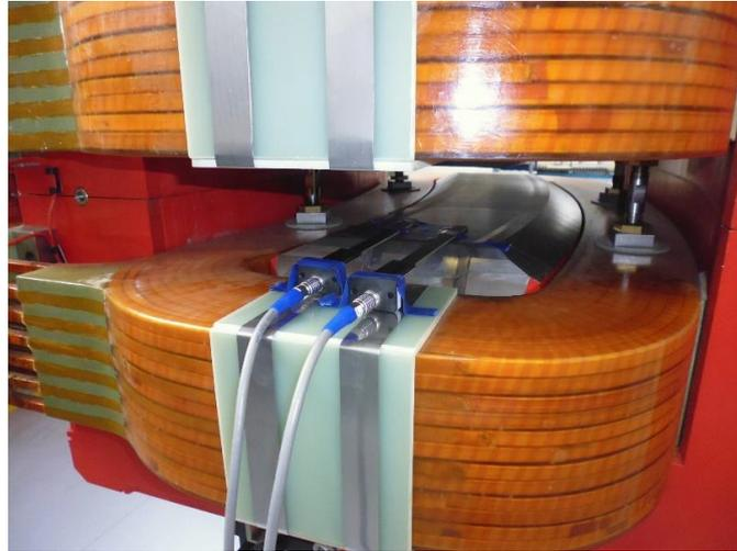
**Figure 6.** The remnant field of the dipole magnet is measured by Hall probe system.
