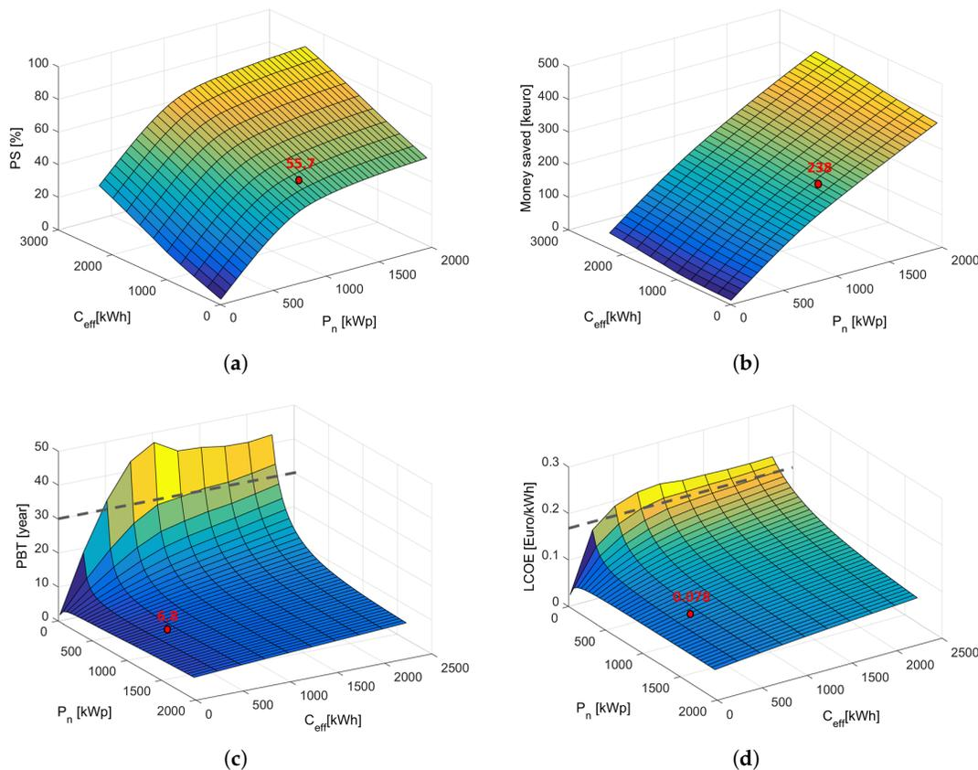
**Figure 6.** Energetic and economic effect of PEC: (a) Percentage of peak shave with respect to the load (PS); (b) Money saved; (c) Pay-back time (PBT); (d) Levelized cost of energy (LCOE).
