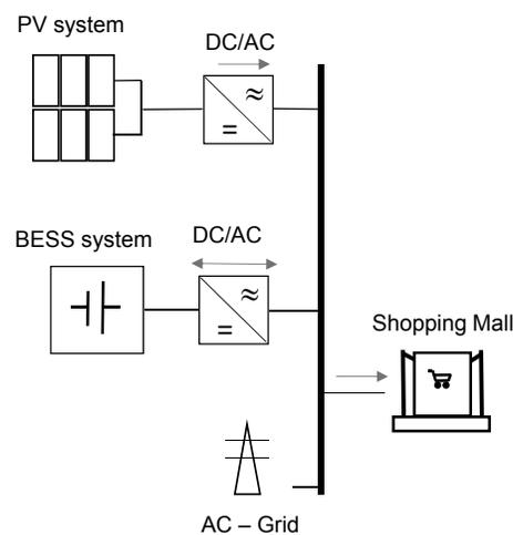
**Figure 1.** Simplified system model composed by: photovoltaic (PV) and battery energy storage (BES) system, shopping mall and electric grid.
