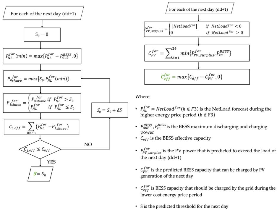
Figure 2. Algorithm for the predictive strategy based on the threshold optimization (on the left) and forecast solar energy to charge the battery energy storage systems (BESS).
