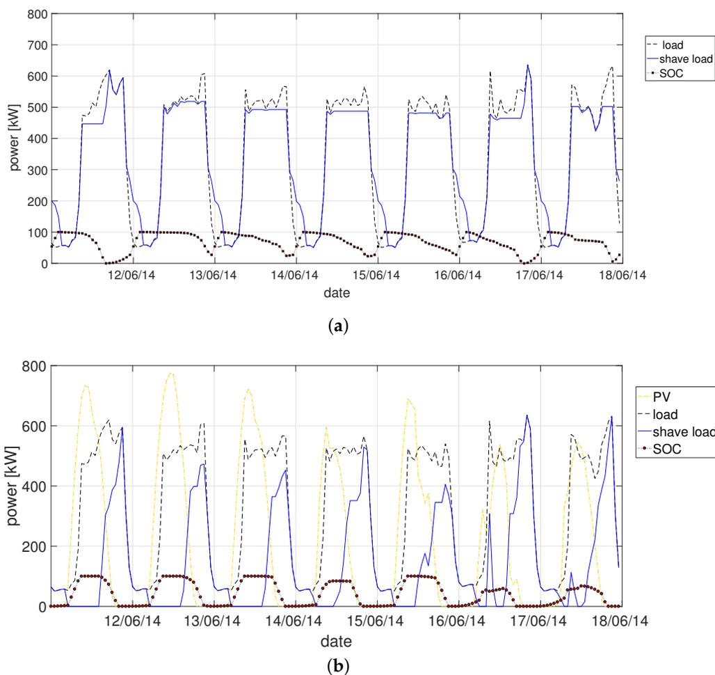
**Figure 7.** Weekly time series of load, shaved load and state of the charge (SOC): (a) With only 500 kWh of BESS; (b) With 500 kWh of BESS and 1000 kWp PV plant.
