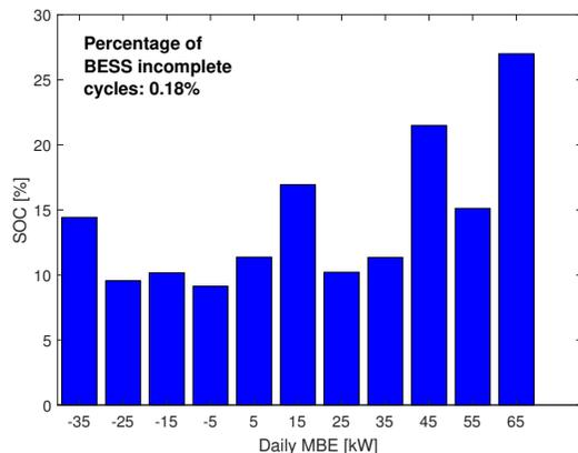
Figure 8. Number of incomplete cycles due to Netload forecast errors (daily mean bias error (MBE)).
