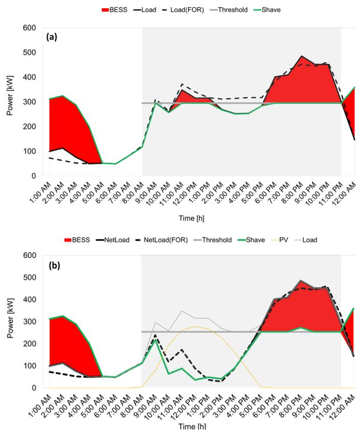
**Figure 4.** Examples of load shaving obtained using the predictive energy control (PEC) strategy: (a) Only BESS is present; (b) Both BESS and PV system are present.
