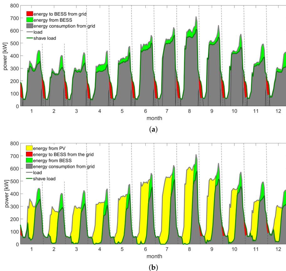
Figure 9. Monthly average of the daily energy and power profiles needed to fulfil the electric demand before and after the peak-shaving: (a) with only 500 kWh of BESS; (b) with 500 kWh of BESS and 1000 kWp PV plant.
