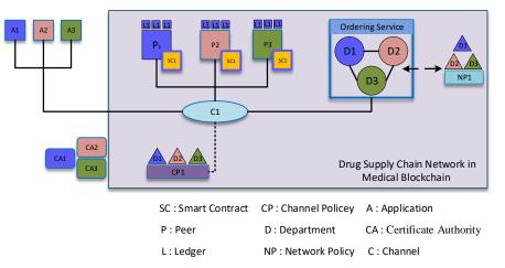
**Figure 8.** Network topology for drug supply chain management based on Hyperledger Fabric in a medical blockchain platform.
