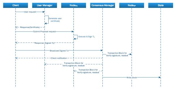
**Figure 7.** Transaction flow in the proposed drug supply chain management in a medical blockchain platform.
