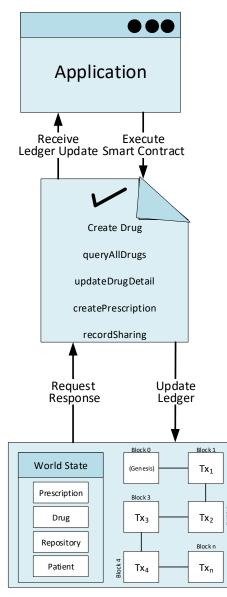
Figure 6. Querying and updating a ledger using a smart contract.
