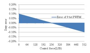
Figure 9. Curves of duty cycle error versus control force for the PWFM strategy.
