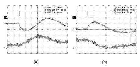
**Figure 18.** Zoom-in waveforms based on the proposed PWFM control strategy: (1) load enable; (2) AC output voltage; (3) inductor current, due to (**a**) from 25% to 75%; (**b**) from 75% to 25%.
