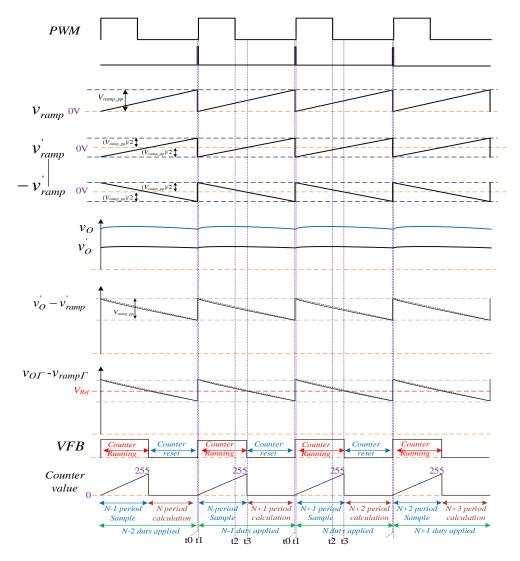
Figure 4. Waveforms relevant to sampling sequence.
