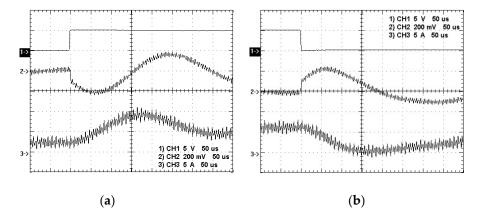
**Figure 16.** Zoom-in waveforms based on the traditional PWM control strategy: (1) load enable; (2) AC output voltage; (3) inductor current, due to (**a**) from 25% to 75%; (**b**) from 75% to 25%.
