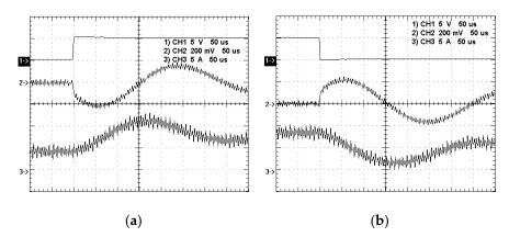
**Figure 19.** Zoom-in waveforms based on the proposed PWFM control strategy: (1) load enable; (2) AC output voltage; (3) inductor current, due to (a) from 50% to 100%; (b) from 100% to 50%.
