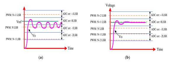
**Figure 1.** Quantization resolution in a digitally controlled pulse width modulation (PWM): (**a**) with limit cycle oscillation; (**b**) without limit cycle oscillation.
