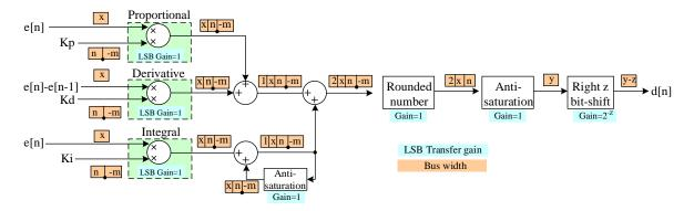
Figure 7. Proportional-integral-derivative (PID) compensator block diagram.
