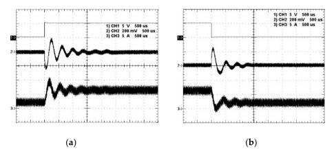
**Figure 14.** Waveforms based on the proposed PWFM control strategy: (1) load enable; (2) AC output voltage; (3) inductor current, due to (**a**) from 25% to 75%; (**b**) from 75% to 25%.
