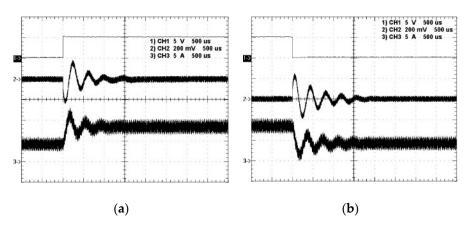
**Figure 15.** Waveforms based on the proposed PWFM control strategy: (1) load enable; (2) AC output voltage; (3) inductor current, due to (**a**) from 50% to 100%; (**b**) from 100% to 50%.
