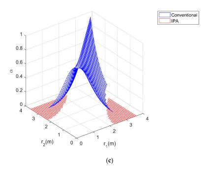
**Figure 5.** Simulation results for Scenario 1 based on the proposed adaptive power allocation scheme, gain ratio power allocation (GRPA) scheme, and IPA scheme, respectively: (**a**) total achievable data rate; (**b**) user fairness; (**c**) optimal power allocation factor.
