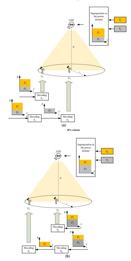
**Figure 2.** NOMA-VLC system based on different power allocation schemes: (**a**) conventional power allocation scheme; (**b**) inverse power allocation (IPA) scheme.
