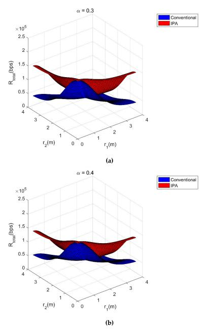
**Figure 3.** Total achievable data rate in conventional power allocation case and IPA case when: (a)  $\alpha = 0.3$ ; (b)  $\alpha = 0.4$ .
