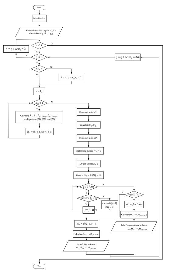
Figure 4. Flow chart of the proposed adaptive power allocation scheme.
