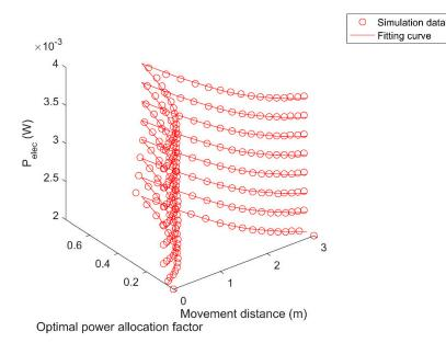
**Figure 10.** Optimal power allocation factor versus movement distance under different  $P_{\text{elec}}$  values.
