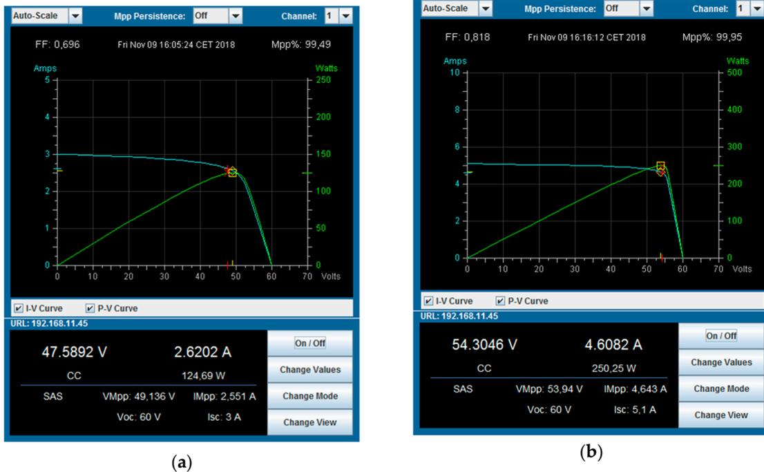
Figure 8. MPP tracking measurements for input power of 124 W (a) and 250 W (b).
