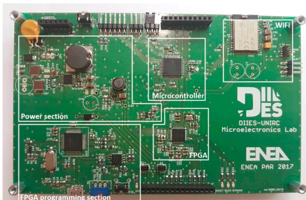
Figure 4. Main logic board top view.
