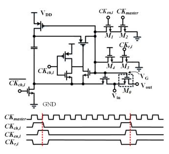
Figure 3. Channel-selection-embedded bootstrap switch.
