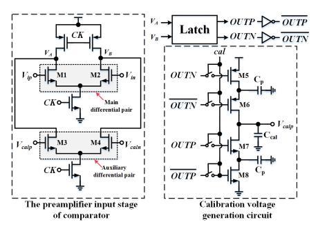
Figure 5. The diagram of comparator's background offset calibration.
