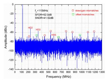
Figure 9. Output fast Fourier transform (FFT) spectrum.
