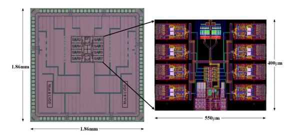
Figure 7. Die micrograph with layout view.
