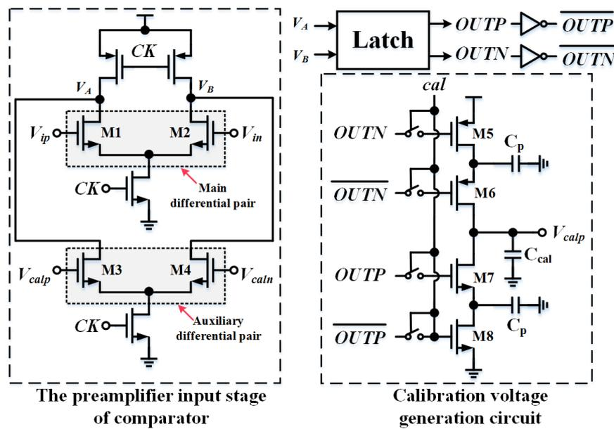
Figure 5. The diagram of comparator's background offset calibration.
