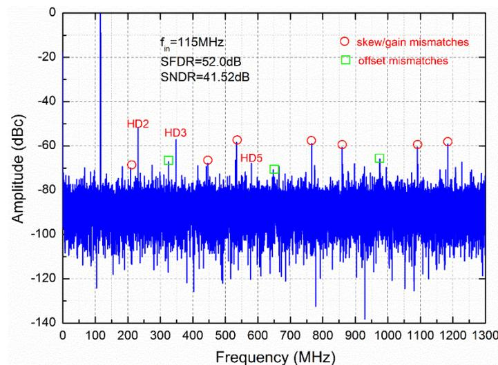
**Figure 9.** Output fast Fourier transform (FFT) spectrum.
