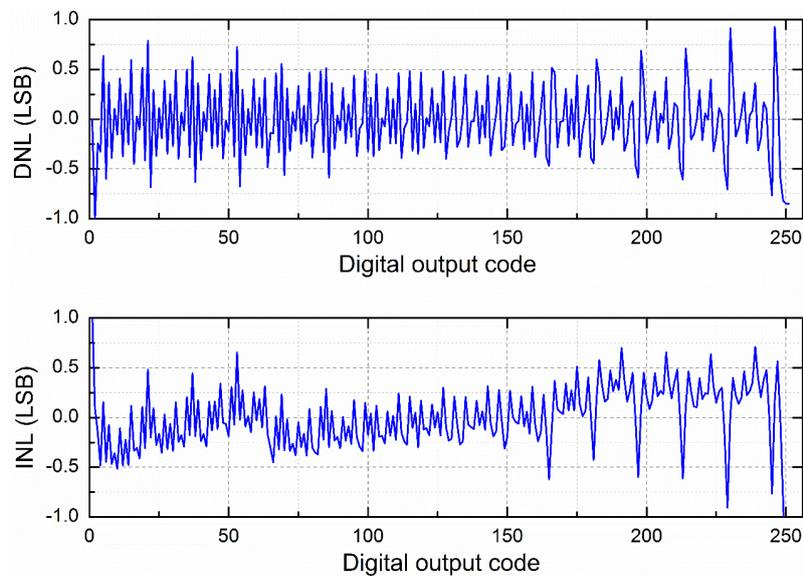
**Figure 8.** Measured differential non-linearity (DNL) and integral non-linearity (INL).
