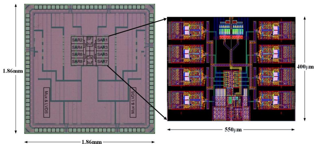
Figure 7. Die micrograph with layout view.
