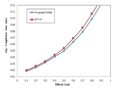
**Figure 10.** Average completion time comparison between EFT-VF and our proposed DWBA at a 10-Gbps data rate per channel.
