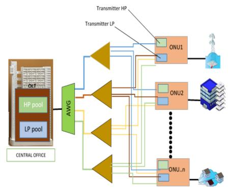
Figure 4. NG-EPON architecture for the proposed DWBA. LP, low priority; HP, high priority.
