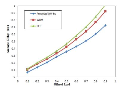
**Figure 5.** Average packet delay of different DWBA Algorithms with a 1-Gbps data rate for each channel. WBM, weighted bipartite matching; EFT, earlier finished time.
