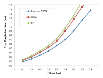
Figure 6. Average completion time of different DWBA algorithms with a 1-Gbps data rate for each channel.
