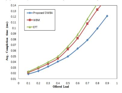
Figure 8. Average completion time of different DWBA algorithms with a 10-Gbps data rate for each channel.
