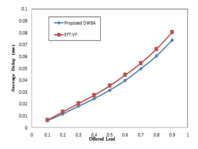
**Figure 9.** Average packet delay comparison between EFT void filling (VF) and our proposed DWBA at a 10-Gbps data rate per channel.
