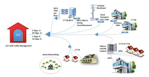
Figure 1. Next-generation EPON. ONU, optical network unit; OLT, optical line terminal.
