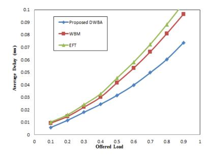
Figure 7. Average packet delay of different DWBA algorithms with a 10-Gbps data rate for each channel.
