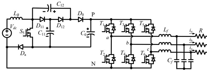
Figure 7. Proposed three-phase VMC-qSBI in simulation.
