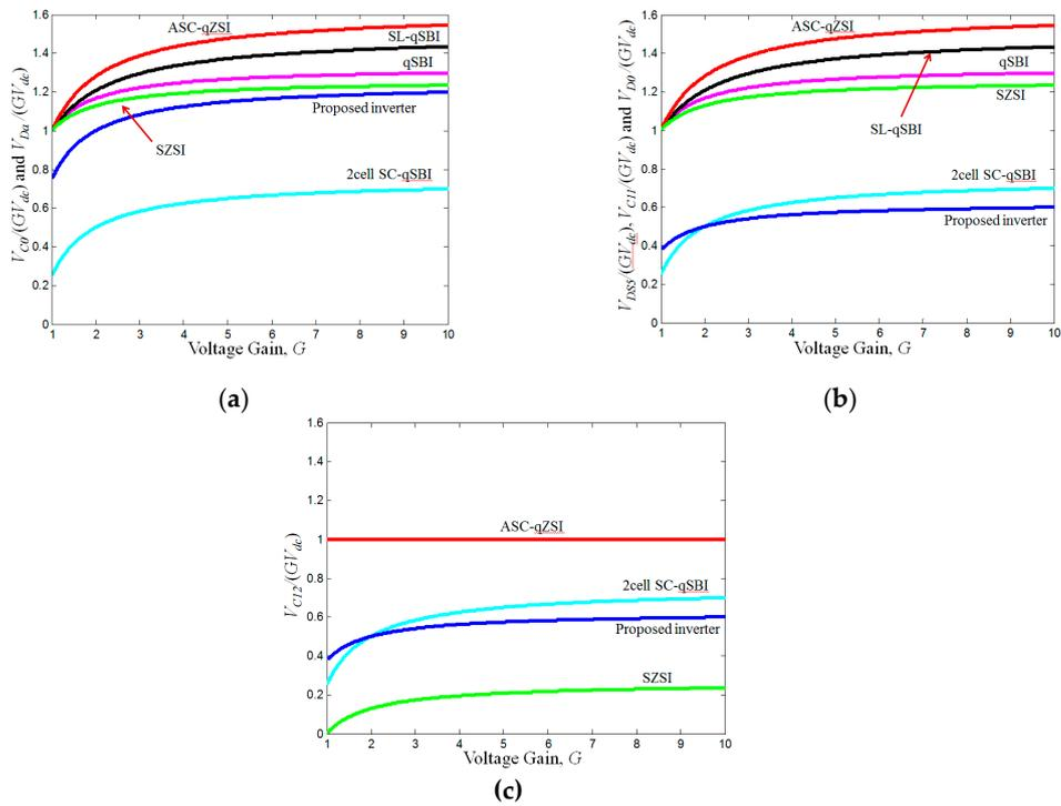
**Figure 4.** Voltage stress comparison. (a) Voltage stress on capacitor  $C_0$  and diode  $D_a$ , (b) voltage stress on switch  $S_5$ , capacitor  $C_{11}$ , and diode  $D_0$ , and (c) capacitor  $C_{12}$  voltage stress.
