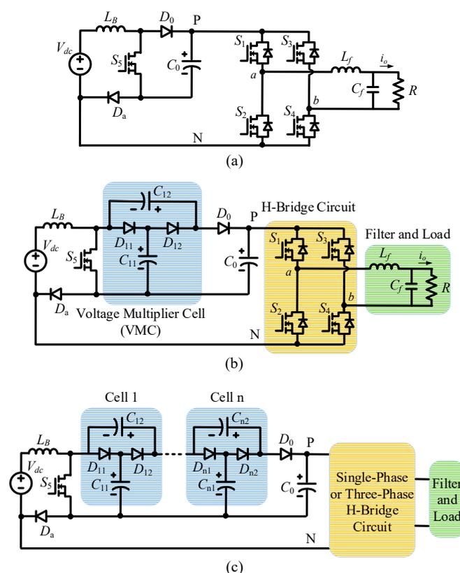
**Figure 1.** Conventional and proposed inverter topologies. (a) Conventional quasi-switched boost inverter (qSBI), (b) proposed single voltage multiplier cell (VMC-qSBI), and (c) proposed  $n$ -VMC-qSBI extension topologies.
