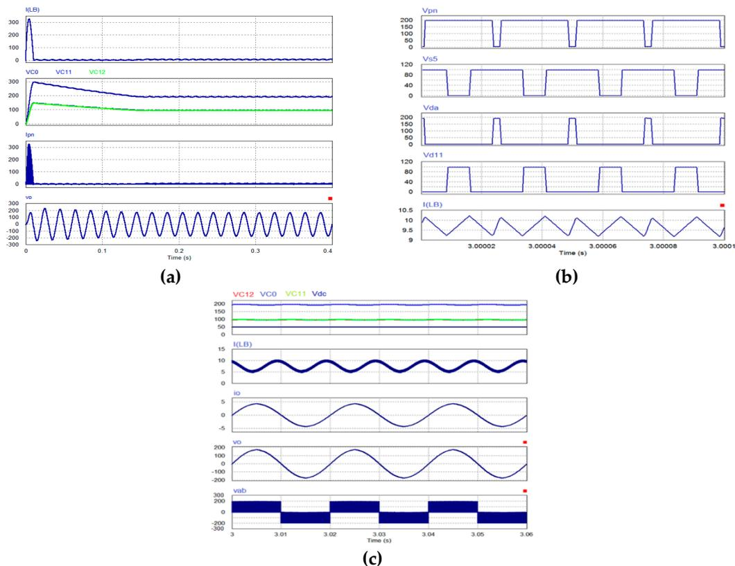
**Figure 6.** Simulation results for the proposed single-phase VMC-qSBI when  $V_{dc} = 50$  V. From top to bottom: (a) input current, capacitor voltages, dc-link current, and output voltage; (b) dc-link voltage, drain-source voltage of  $S_5$ , diodes  $D_a$ – $D_{11}$  voltage, and input current; and (c) input voltage and capacitors voltages, input current, output current, and output voltages before and after the L-C filter.
