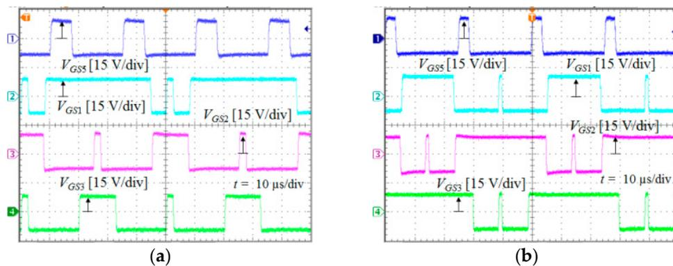
**Figure 11.** Control signal waveforms when (a)  $V_{dc} = 50$  V and (b)  $V_{dc} = 72$  V.
