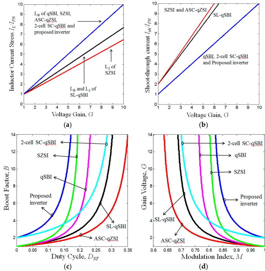
**Figure 5.** Voltage and current stress comparison. (a) Inductor current stress, (b) ST current stress, (c) boost factor, and (d) voltage gain.
