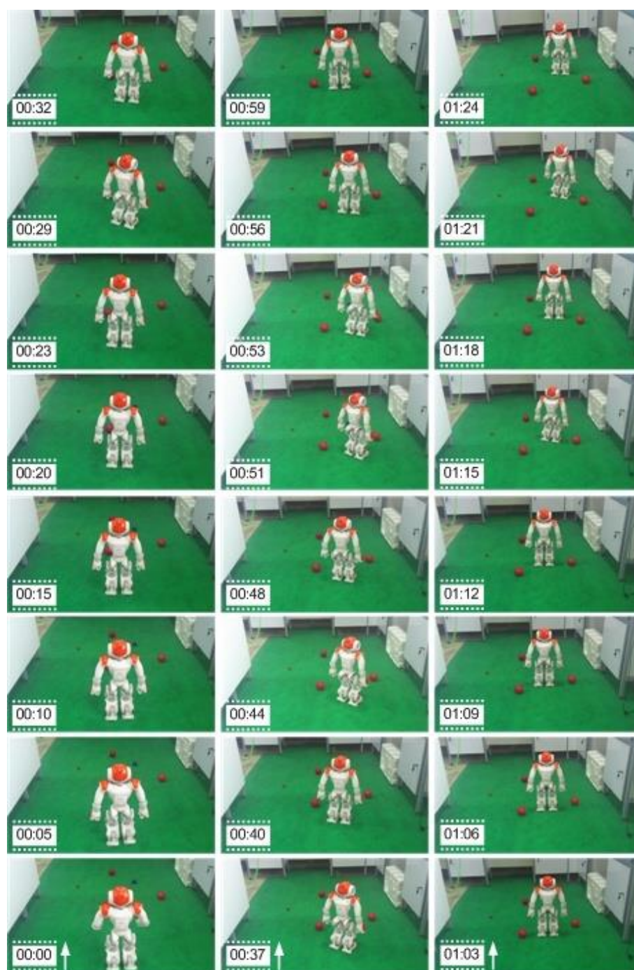
Figure 8. The path traversed by the Nao humanoid robot using the linguistic method (see the video of the robot's movement).
