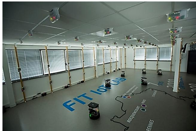
**Figure 4.** Lille-testbed network grid over ceiling and wooden poles in Inria building floors.
