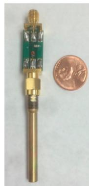
**Figure 13.** Picture of EIMN with an ultrasonic transducer showing the printed circuit board (PCB) implemented with shunt capacitor of 100 pF and series inductor of 8 nH. Reproduced with permission from Reference [41], Copyright Elsevier, 2016.
