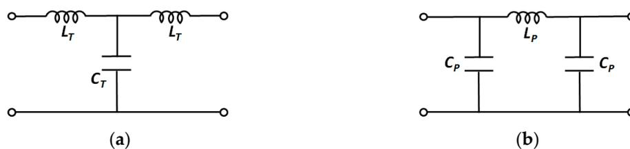
Figure 5. Impedance matching networks for cables (a) T-type and (b)  $\Pi$ -type [95].
