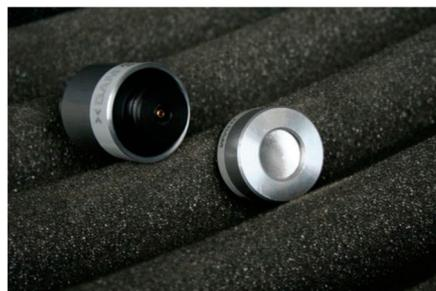
**Figure 17.** Focusing transducer based on cellular polypropylene with an electric matching unit shown in the background for air-coupled ultrasonic testing. Reproduced with permission from Reference [151], Copyright AIP, 2016.
