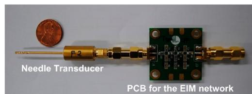
**Figure 15.** Needle ultrasonic transducer with filter based electric impedance matching network. Reproduced with permission from Reference [120], Copyright Elsevier, 2016.
