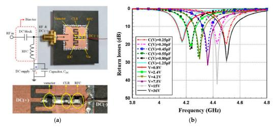
**Figure 1.** (a) Fabricated prototype of the reconfigurable antenna and (b) its frequency response for different voltage values [20]. Reproduced with permission from [20], Copyright IEEE, 2014.
