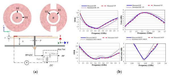
**Figure 4.** (a) Schematic and (b) standing wave ratio (SWR), gain, and axial ratio characteristics of the antenna [44]. Reproduced with permission from [44], Copyright IEEE, 2017.
