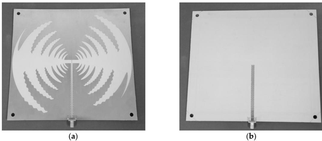
Figure 8. Both sides of the produced sinuous slot antenna with a CPWG excitation: (a) top, (b) bottom.
