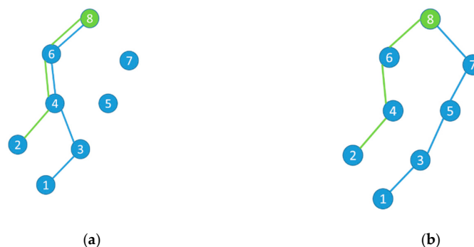
Figure 5. Depicts the routing paths for the traffic generated by nodes 1 and 2, in green and blue colors, respectively. (a) Demonstration of a possibility for overloading nodes 4 and 6 while routing the traffic to node 8, where (b) shows a more balanced traffic distribution among the nodes.
