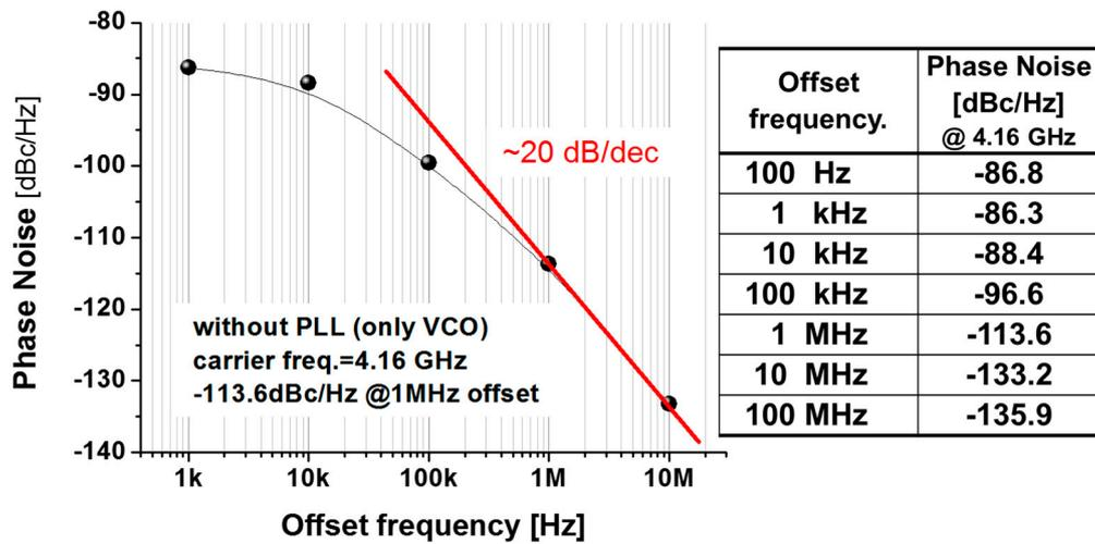
Figure 4. Measured phase noise with offset frequency.
