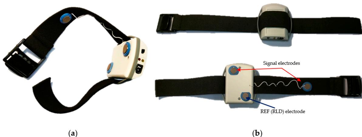
**Figure 7.** Arm-ECG sensor system WAMECG1: (a) prototype assembly; (b) top and bottom views of the system.
