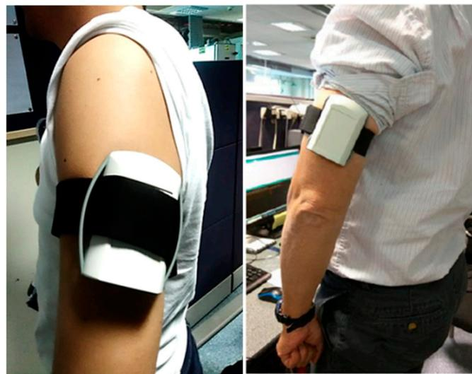
**Figure 21.** Photos of the devised arm-ECG sensor prototype (WAMECG1) being worn by volunteers.
