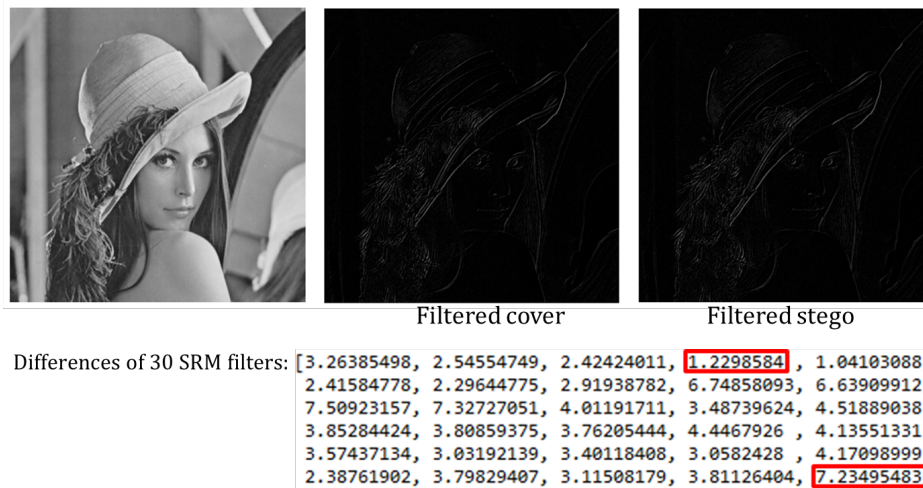
Figure 14. Selection of more effective SRM filters: a large difference (e.g., 1.229 and 7.234) depending on the filter between the filtered cover and stego images is found after each SRM filter is applied.
