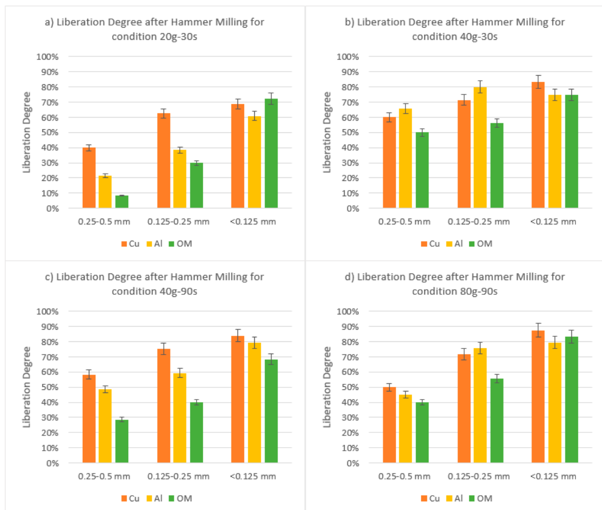
Figure 4. Degree of liberation determined by the SEM-EDS image analysis. (a) Feed = 20 g, Milling Time = 30 s; (b) Feed = 40 g, Milling Time = 30 s; (c) Feed = 40 g, Milling Time = 90 s; (d) Feed = 80 g, Milling Time = 90 s.
