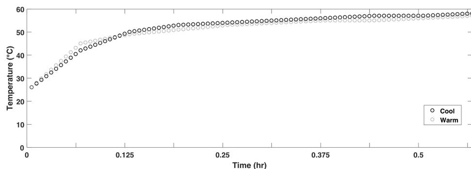
**Figure 3.** The mean values of the junction temperature of the cool channel (black) and warm channel (gray) of the LED light source increasing as a function of time.
