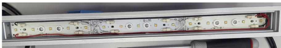
**Figure 4.** The Laser Blade is based on 7 cool Correlated Color Temperature (CCT) LEDs and 8 warm CCT LEDs positioned alternately with each other.
