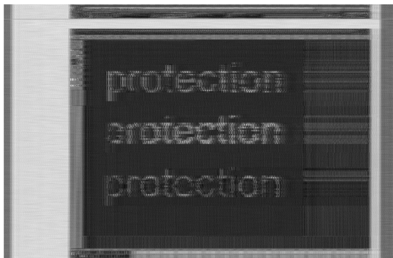
Figure 17. An example of an image obtained based on compromising emanations measured in the frequency f_0 = 642 MHz ( BW = 100 MHz, sampling frequency f_s = 250 MHz).
