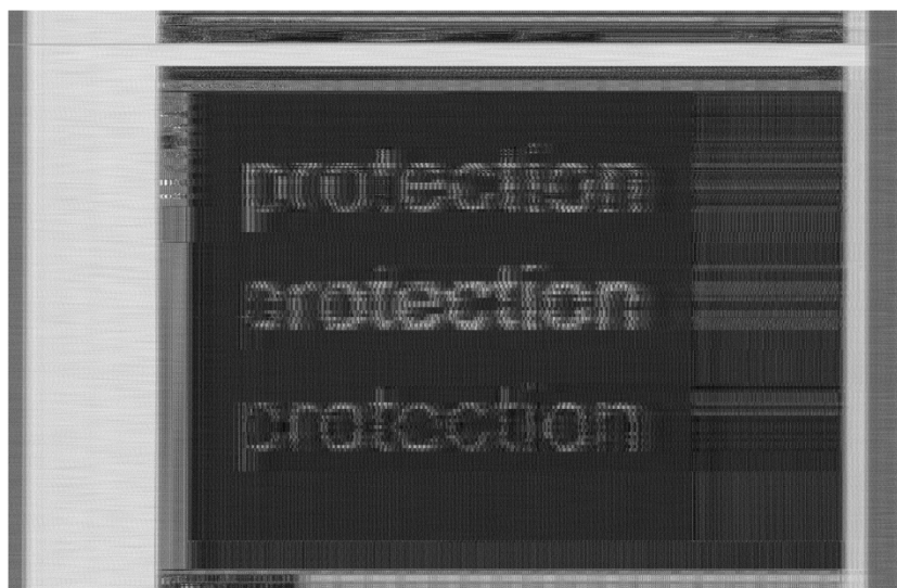
Figure 17. An example of an image obtained based on compromising emanations measured in the frequency f_o = 642 MHz ( BW = 100 MHz, sampling frequency f_s = 250 MHz).
