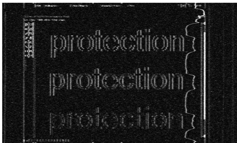
Figure 18. An example of an image obtained based on compromising emanations measured in the frequency f_0 = 494 MHz ( BW = 10 MHz, sampling frequency f_s = 1250 MHz) for a source of emission in analogue VGA standard form.
