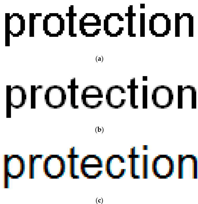
Figure 4. Application effects of edge smoothing modes of graphic characters in Windows XP OS: (a) without edge smoothing mode (inaccessible for Windows 7 OS), (b) Standard edge smoothing mode, and (c) ClearType edge smoothing mode.
