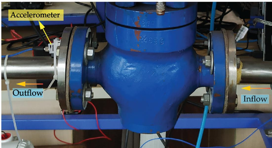
Figure 5. Placement of accelerometer to capture vibration signal.
