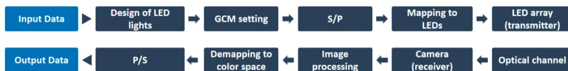
**Figure 12.** GCM-based visual MIMO transceiving process including the design of LED lights [26].
