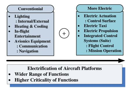
Figure 1. Increased use of electrical power in a more electric aircraft (MEA).
