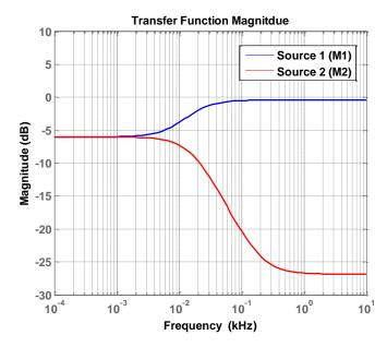
Figure 8. Frequency response of transfer functions for source 1 and source 2.
