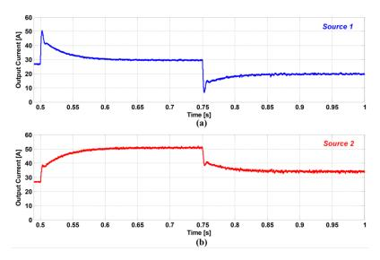
**Figure 15.** Simulation results of the proposed approach with step-up/step-down changes. (**a**): Source 1 Output Current, (**b**): Source 2 Output Current.
