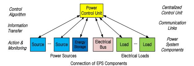
Figure 4. Centralized control architecture for an aircraft EPS.
