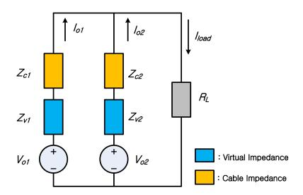
Figure 7. Equivalent circuit of an EPS with two sources connected in parallel.
