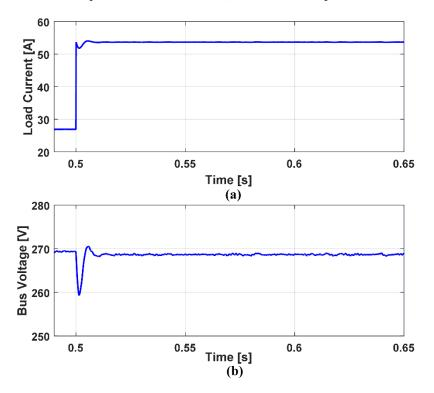
**Figure 12.** Simulated load current and bus voltage ( $L_{v2} = 1 \text{ mH}$ ). (a): Load Current, (b): Bus Voltage.
