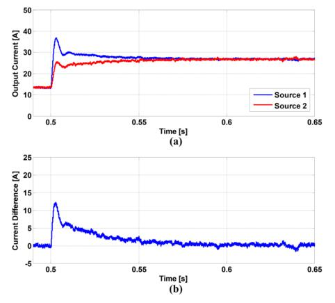
**Figure 11.** Simulated output current waveform ( $L_{v2} = 1$  mH). (a): Output Current, (b): Difference.
