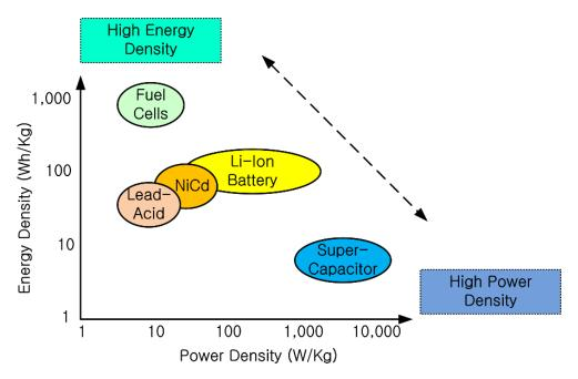
Figure 3. Comparison of power source characteristics (Redrawn using data of [42,43]).
