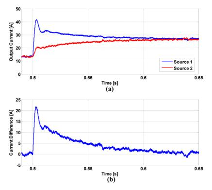
**Figure 13.** Simulated output current waveform ( $L_{v2}$  = 3 mH). (a): Output Current, (b): Difference.
