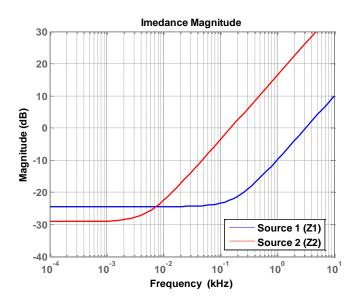
Figure 9. Frequency characteristics of impedances for source 1 and source 2.
