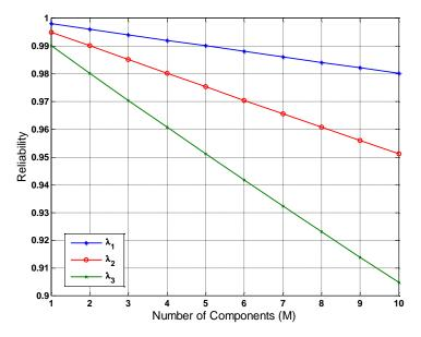
Figure 5. System reliability with different failure rates and number of components.
