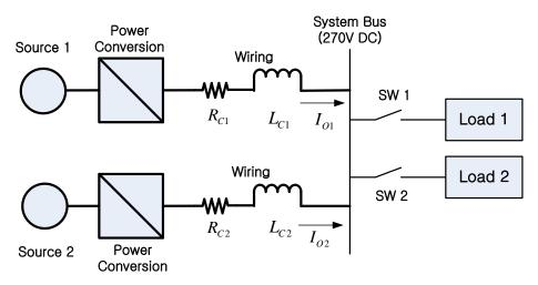
Figure 10. Configuration of the simulated EPS.
