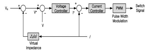
Figure 6. Block diagram of a virtual impedance-based power management.
