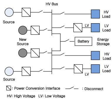
Figure 2. Configuration of a generalized EPS in an MEA.
