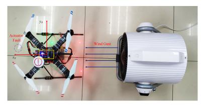
Figure 13. Experimental setup of the quadrotor hovering in the wind field in Case B.
