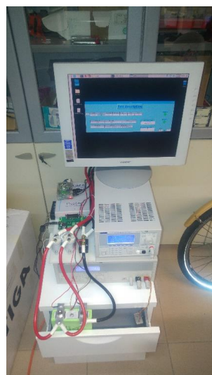
Figure 8. Cell Station Tester experimental setup.
