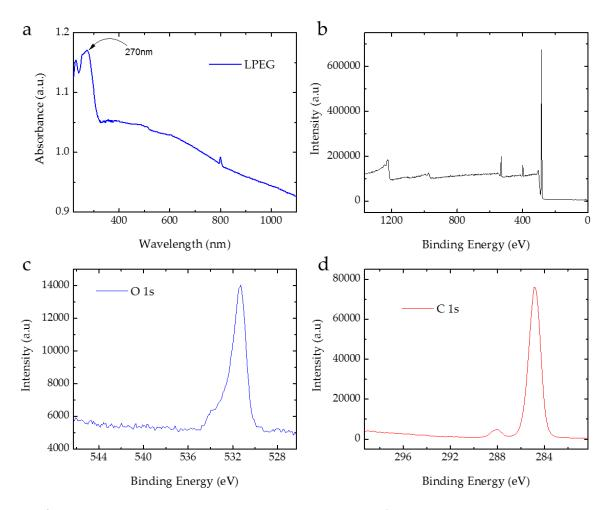
**Figure S1.** (**a**) UV-VIS absorbance spectroscopy of LPEG, (**b**) XPS analysis survey scan, (**c**) O 1s scan, and (**d**) C 1s scan.
