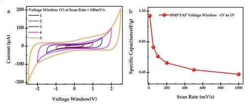
**Figure S2.** (**a**) Cyclic voltammetric plot for bulk graphite powder in BMP-FAP, and (**b**) the resulting specific capacitance vs scan rate used.
