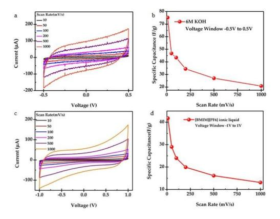
**Figure S3.** (a) Cyclic voltammetric plot of LPE graphene in 6M KOH aqueous electrolyte, and (b) the resulting specific capacitance vs scan rate used. (c) Cyclic voltammetric plot of LPE graphene in BMIM-PF6 ionic liquid electrolyte, and (d) the resulting specific capacitance vs scan rate used.
