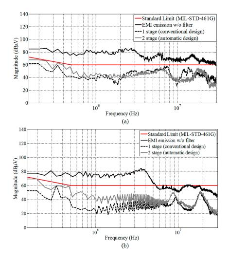
Figure 7. Measured EMI with and without EMI filters (a) case study #1; (b) case study #2.
