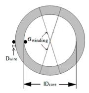
Figure 2. Toroidal core: geometric parameters for Equation (3).
