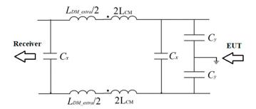
**Figure 5.** Γ-Π filter topology (single stage) for the experimental setup.
