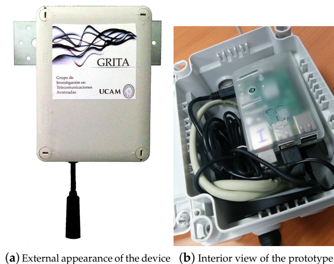
Figure 5. Views of the physical prototype built. (a) Final design of the acoustic device. In the picture, the Raspberry Pi and the other components are inside a protected box. At the bottom part of the box, the microphone can be observed; (b) Interior view of the waterproof case. The components inside of it are the Raspberry Pi together with the POE splitter, the microphone at the bottom of the picture and all the cables for the connection.
