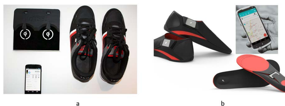
Figure 5. (a) Wiisel footwear system for fall risk application; and (b) Lechal system ® for by Ducere Technologies Pvt. Ltd. (Secunderabad, Andhra Pradesh, India).
