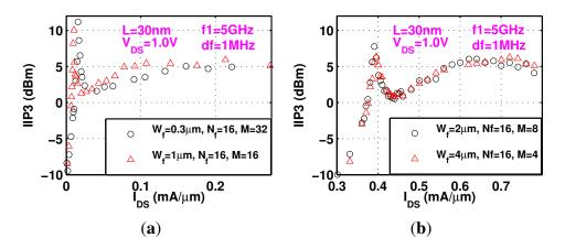
Figure 8. Measured width impact on IIP3. (a) Measured IIP3 at 5 GHz for two 30 nm devices with different total width; (b) Measured IIP3 as a function of  $V_{GS}$  for two 30 nm devices with same total width.
