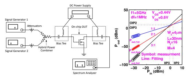
Figure 2. (a) Measurement setup and (b) extrapolation illustration for *IP*3 and *IP*2.
