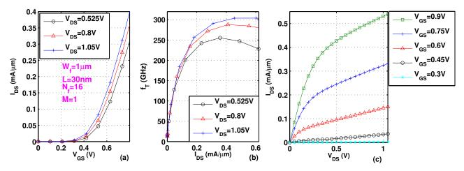
Figure 1. Measured (a)  $I_{DS}$  versus  $V_{GS}$ ; (b)  $f_T$  versus  $I_{DS}$  and (c)  $I_{DS}$  versus  $V_{DS}$ .
