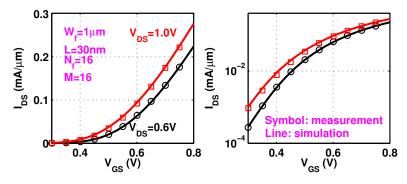
**Figure 5.** Comparison of simulated  $I_{DS}$  versus  $V_{GS}$  with measurement on (**a**) linear and (**b**) log  $I_{DS}$  scales at  $V_{DS} = 0.6$  and 1.0 V.
