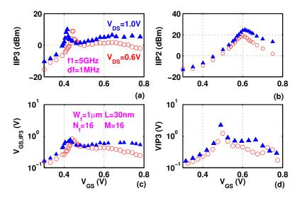
Figure 7. Measured (a) IIP3; (b) IIP2 and (c)  $V_{GS,IP3}$  and (d) VIP3 as a function of  $V_{GS}$  for different  $V_{DS}$ .
