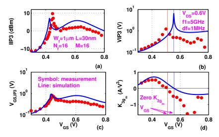
**Figure 6.** (a) *IIP*3 (b) *VIP*3 (c)  $V_{GS,IP3}$  and (d)  $K_{3_{g_m}}$  as a function of  $V_{GS}$  at  $V_{DS} = 0.6$  V.
