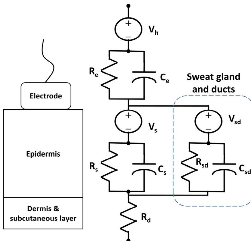
**Figure 4.** Electrical model of electrode-skin interface for electrodermal measurements.
