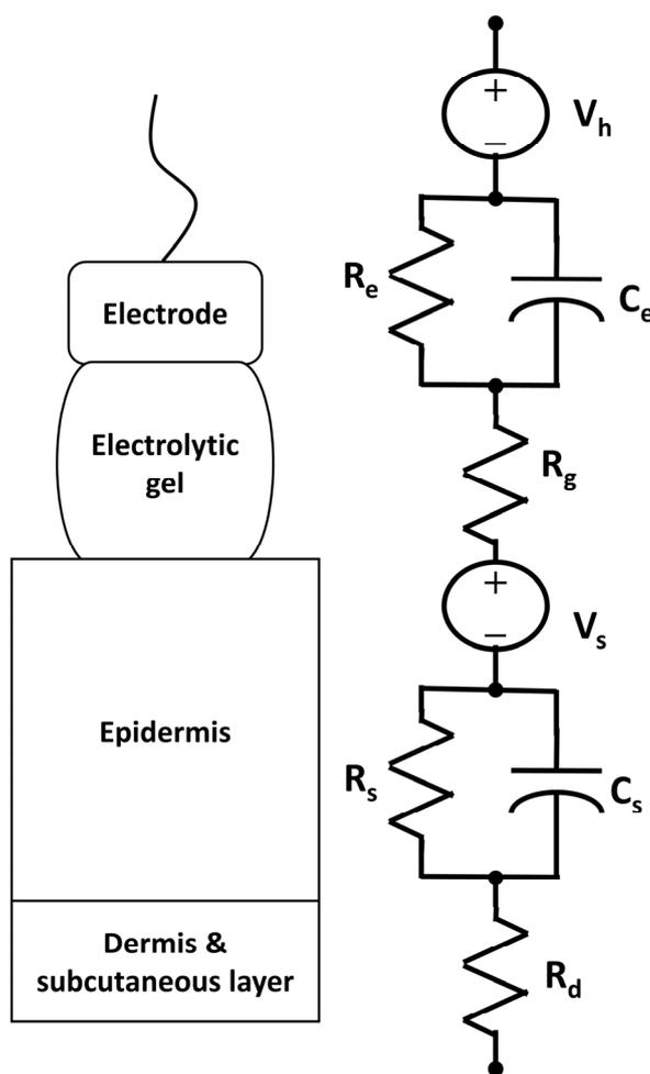
**Figure 2.** Electrical model of biopotential measurement at the skin surface.
