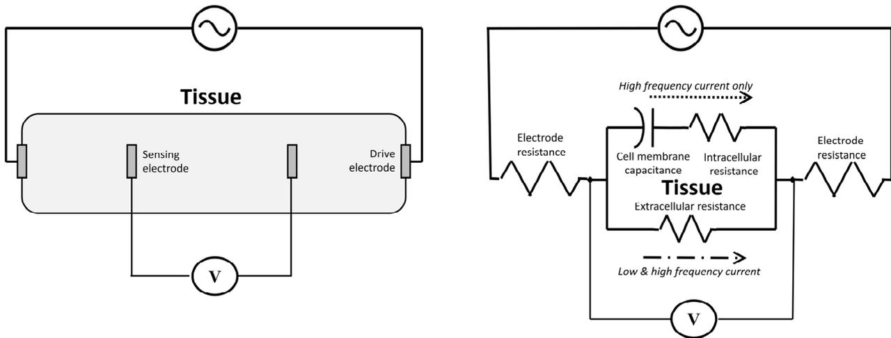
**Figure 3.** Tetrapolar measurement of tissue impedance (**left**); and equivalent electric circuit model (**right**).
