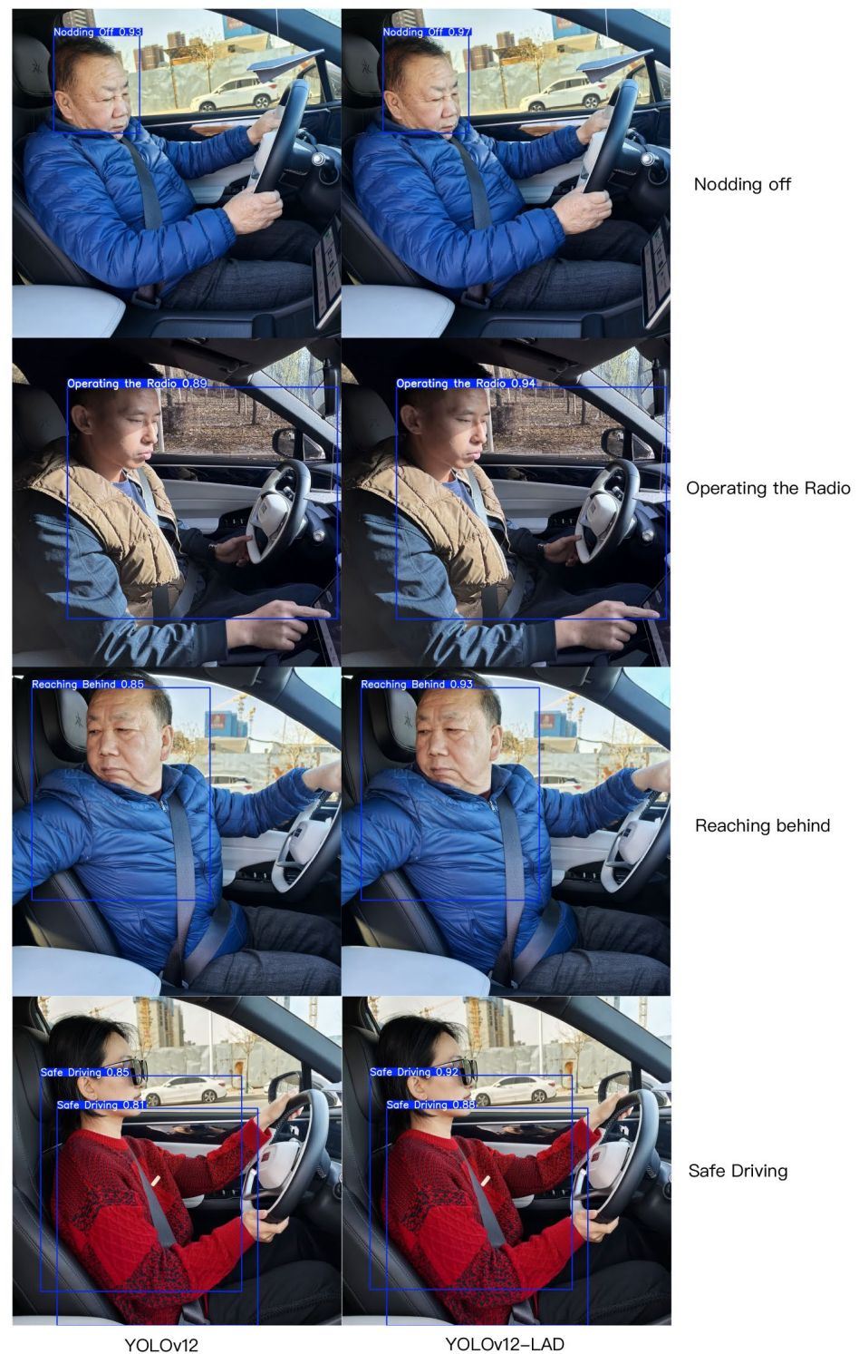
Figure 17. Detection results for the next four distracted driving behavior categories.
