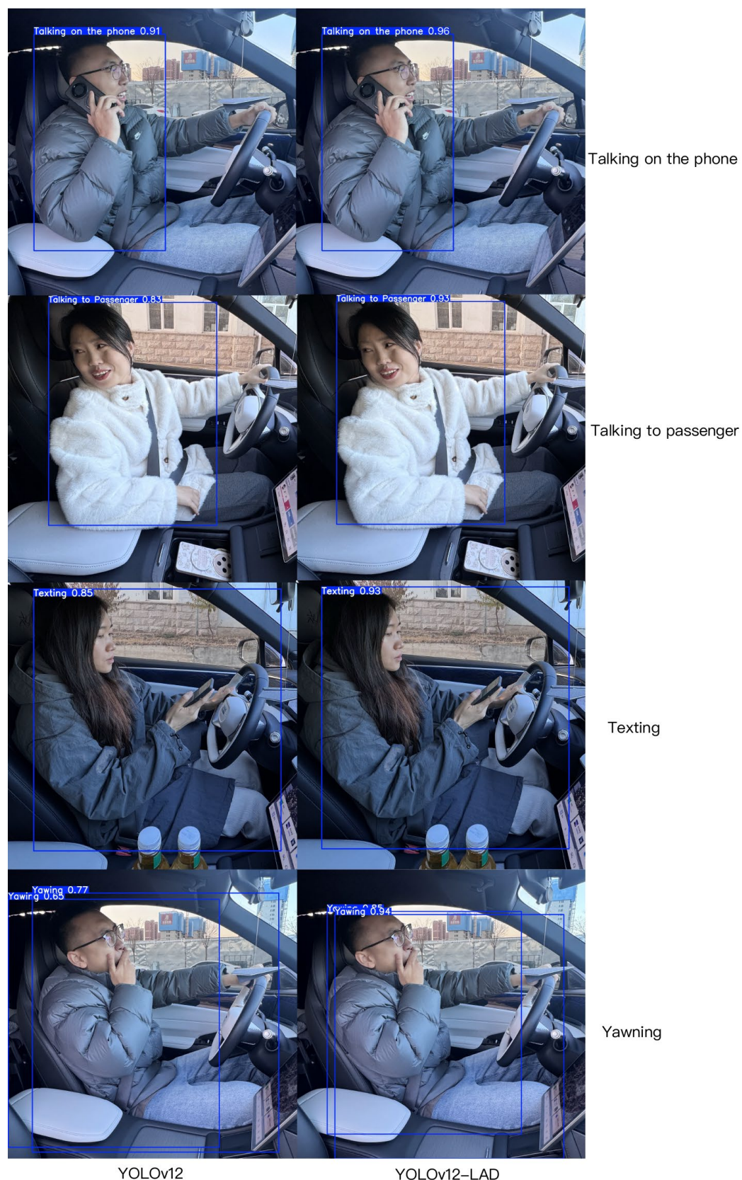
Figure 18. Detection results for the remaining four distracted driving behavior categories.
