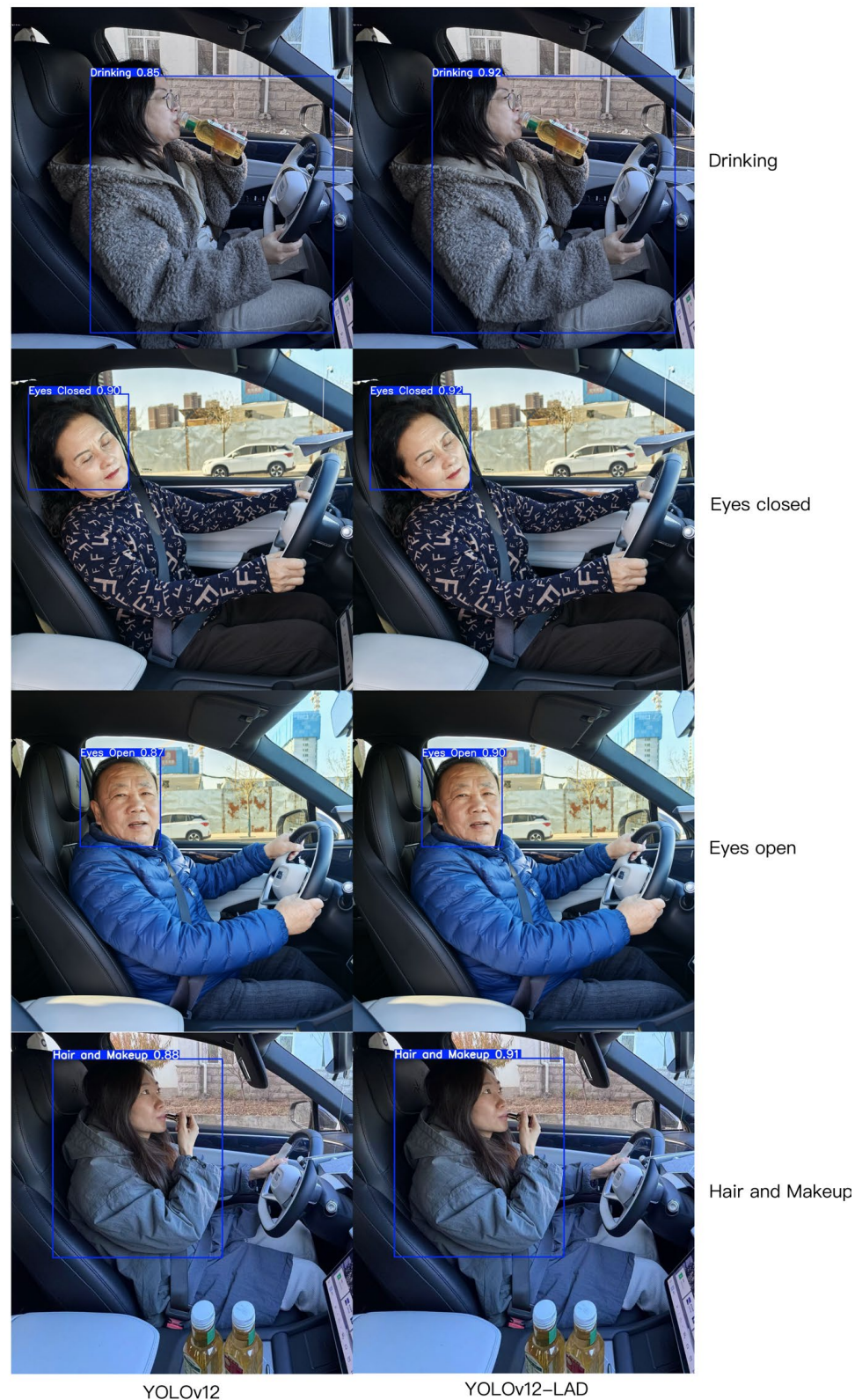
Figure 16. Detection results for the first four distracted driving behavior categories.
