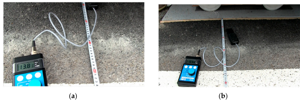
Figure 10. Representative magnetic-flux-density measurements in the occupied area around the realized WPT platform: (a) measurement at 125 mm from the transmitting module, B = 13.8 \mu\text{T} ; (b) measurement at 225 mm from the transmitting module, B = 5.4 \mu\text{T} .
