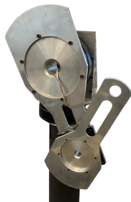
Figure 2. Experimental robot manipulator (the pendulum is the elbow joint).
